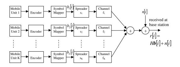
Figure 2.3: The uplink of a *K*-user CDMA system [4].
