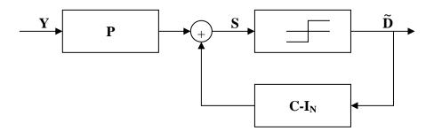
Figure 2.6: Block diagram of BDFE [54].
