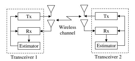
Figure 2.2: Wireless transceiver with channel estimator.
