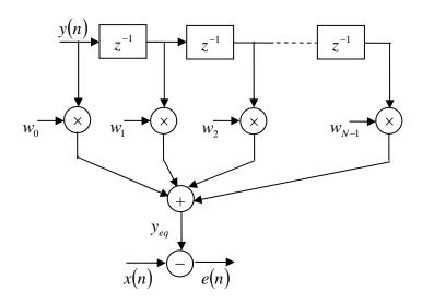
Figure 2.4: Linear Transversal Equalizer (LTE)
