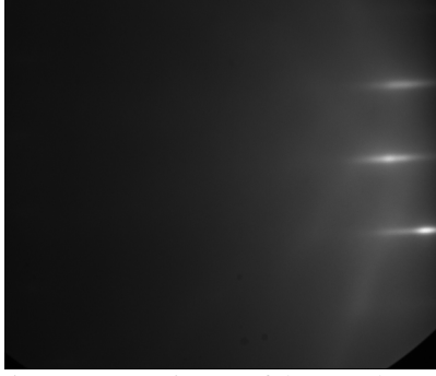
Fig. 4: RHEED image of the GaN layers.
