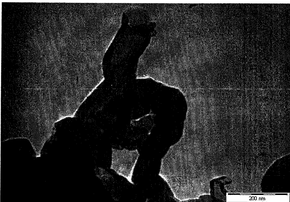
Figure 4: TEM image for purified MWCNTs prepared by preparation method (sol-gel) using oxidation in air followed by sulfuric acid refluxes and re-oxidation in air.
