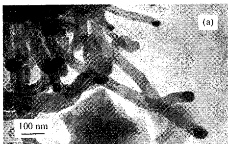
Figure 2. The images of the as-synthesized MWNTs: (a) TEM, (b) SEM
