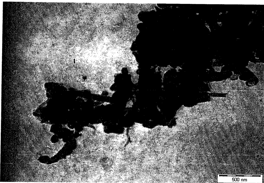
Figure 8: TEM image for purified MWCNTs prepared by different flow rate using oxidation in air followed by sulfuric acid refluxes and re-oxidation in air.
