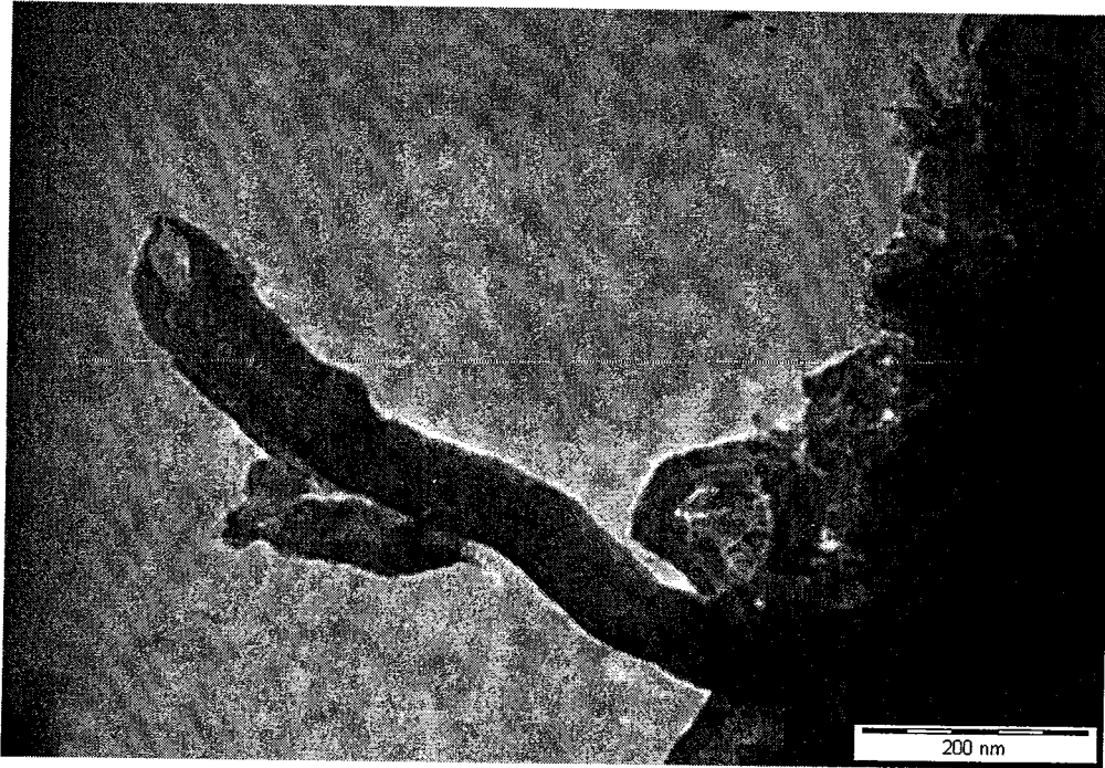
Figure 7: TEM image for purified MWCNTs prepared by different temperature (625 °C) using oxidation in air followed by sulfuric acid refluxes and re-oxidation in air.
