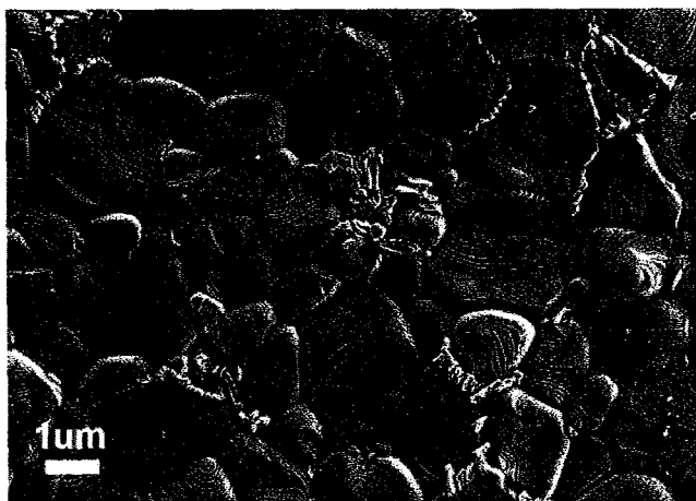
Fig. 3. FESEM image (surface) of MW sintered of CCTO for 120 min. Sample was pre-sintered at 1000 °C/10 h using a conventional furnace.
