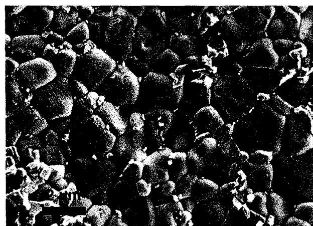
Fig. 6. SEM images of MW treated CCTO for 60 min with selected SnO 2 dopant concentrations of (a) 1 mol%, (b) 4 mol%, and (c) 6 mol%.
