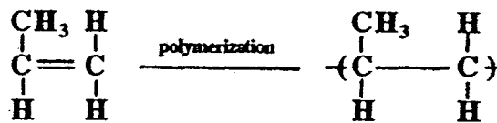
Rajah 1.2.1 Tindakbalas pempolimeran propilena. [Theodore, 1969]
