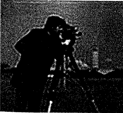
Fig. 5 DCT method compression factor of 16
