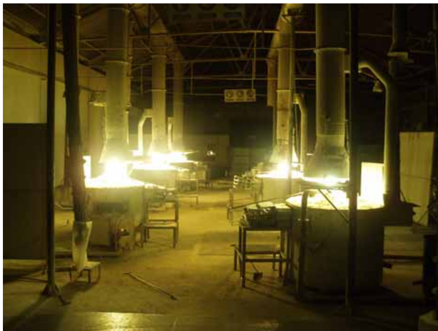
Plate 1.2: Interior of Approit ZnO Manufacturing Sdn Bhd factory showing 5 furnaces that are used to synthesize ZnO nanocrystals for this work.
