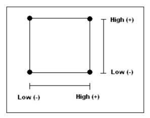
Figure 2.1: The 2<sup>2</sup> factorial design (Source: Myers & Montgomery, 2002)
