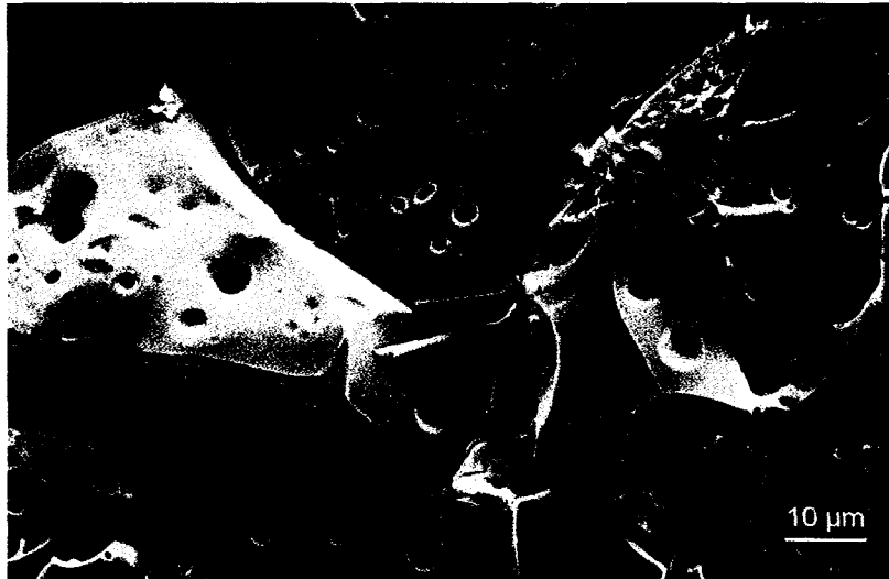
Figure 18. The microstructure of the melt and abnormal grain growth for sample sintered at 1050°C for 24 hours (Mag: 1000X).
