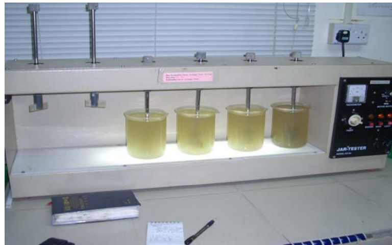
Plate 2.5: Jar testing apparatus (With permission from the Segama WTP)
