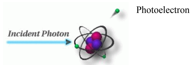
Figure 2.1 Schematic representation of the photoelectric effect. (Taken from Sprawls Educational Foundation)
