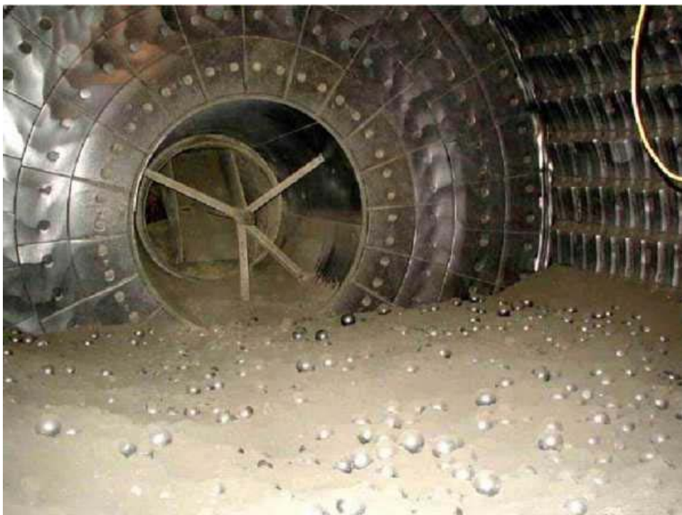
Figure 2.6: Cement mill for grinding clinker and gypsum [Understand Cement, 2002]
