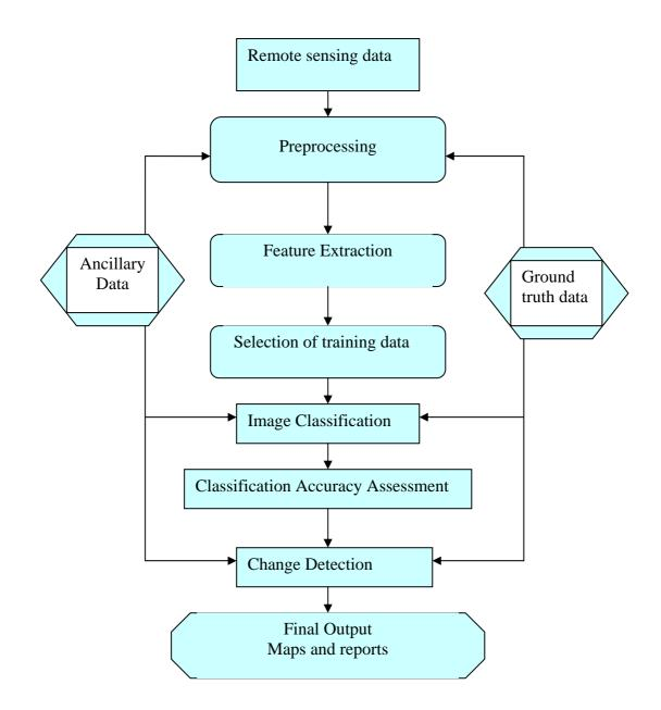
Fig. 1.1 A flowchart of procedure for deriving land use/land cover data and change detection from remotely sensed data.
