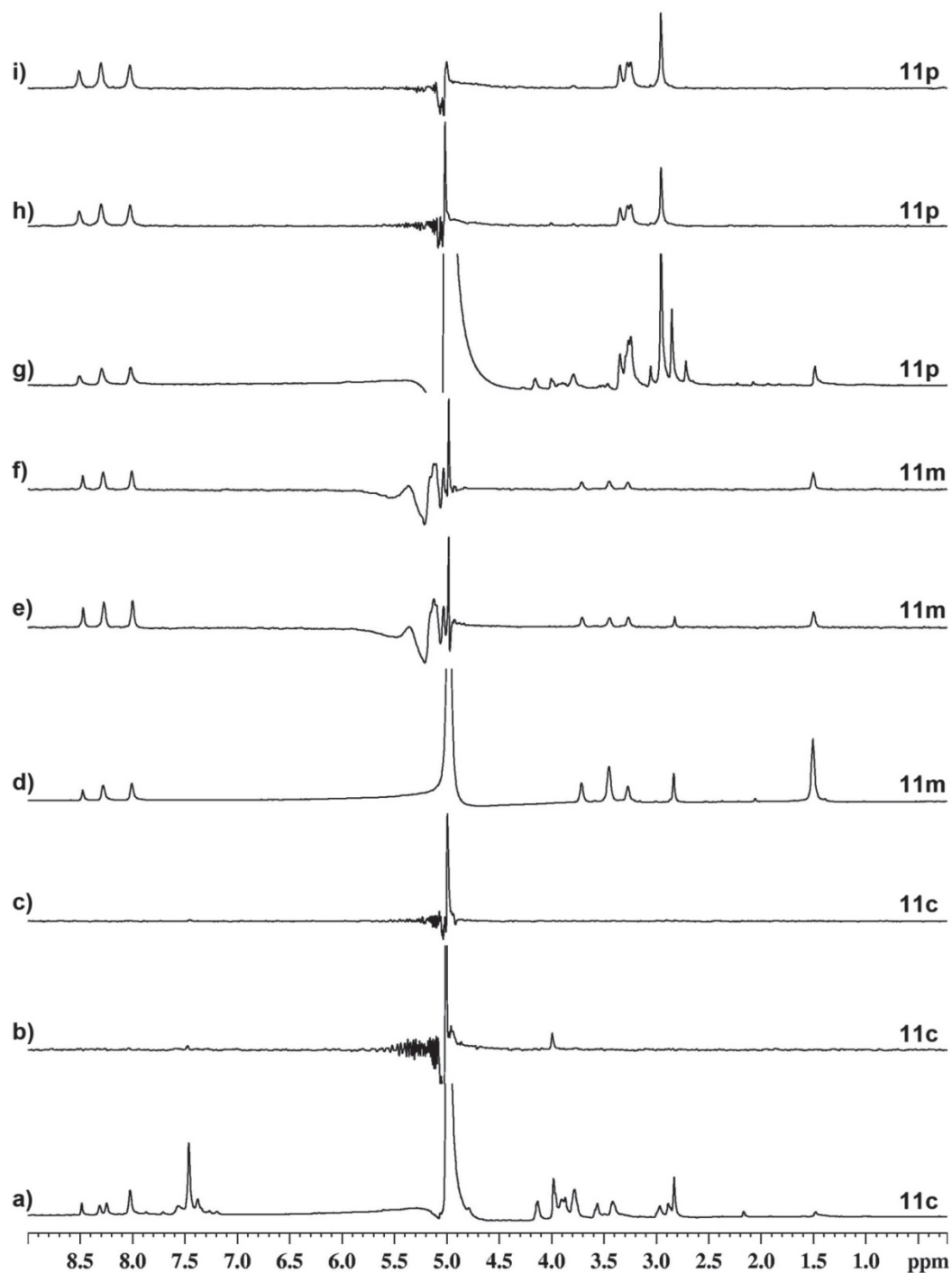
Figure 28. 1D proton spectra (a, d, g) and the corresponding STD NMR spectra recorded upon saturation at 10 ppm (b, e, h) and -1 ppm (c, f, i) of 11c /, 11m /, and 11p /DNA complexes, respectively. The STD NMR spectra were plotted with the same noise level.
