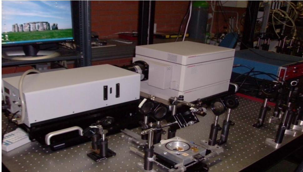
Figure 3.2. The picture shows the spectrometer and streak camera of acquisition setup
