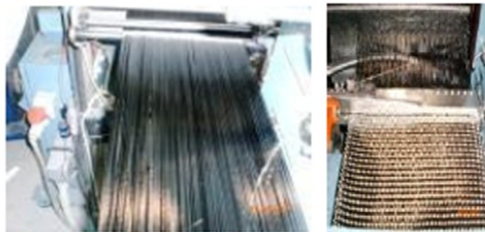
Figure 6- 14: Weaving phases. a) the carbon hybrid yarns input in the loom. b) weft yarn positioning.
