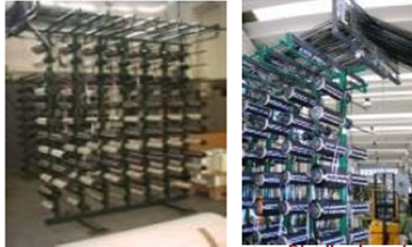
Figure 6- 13: Arrangement of yarns on the weaving creel.
