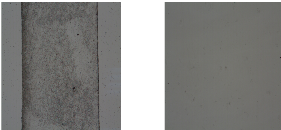
Figure 4.4. Optical photographs of the silicon chips after KOH wet etch: left, a 700 nm etched dig on unprotected crystalline silicon; right, unetched silicon surface protected by the hydrophobin biofilm.
