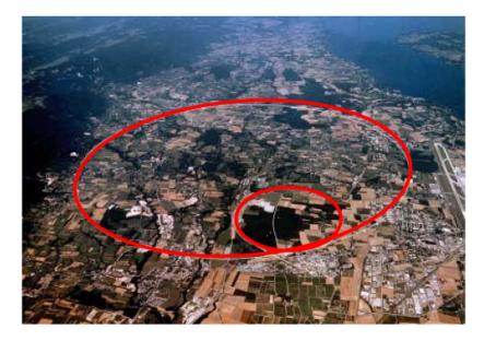
Figure 1.2: Overview of the Geneva area with a drawn of the two circular accelerators: Super Proton Synchrotron (SPS 7 Km) and the Large Hadron Collider (LHC 27 Km).
