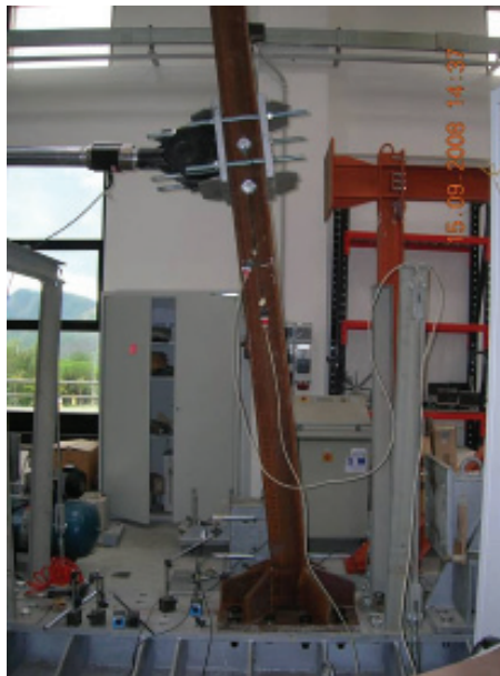
Fig. 43. Adopted set-up of cantilever beam
