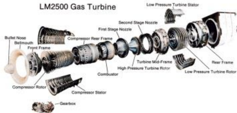
Figure 9.2- LM 2500+ Gas Generator Layout
