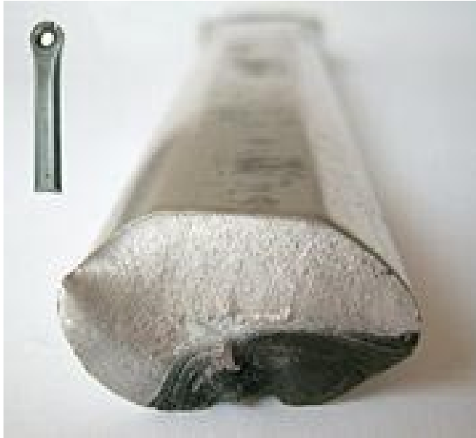
Figure 2.2- Fracture of Inconel Crank Arm. Dark area: slow crack growth. Bright area: sudden fracture.
