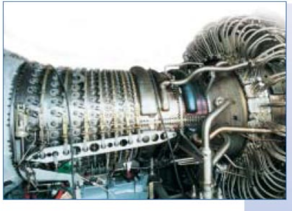
Figure 9.3- LM2500+ Gas Generator
