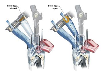
Figure 2.5 Intake and exhaust ducts: swirl index control
