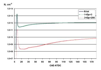
Figure 5.20 - Number concentration of particles in the 1-3nm size range and 3-200nm.
