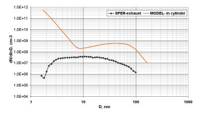
*Figure 5.32* – Number weighted particle size distribution measured by DMA compared with the simulation results at 180 CAD ATDC
