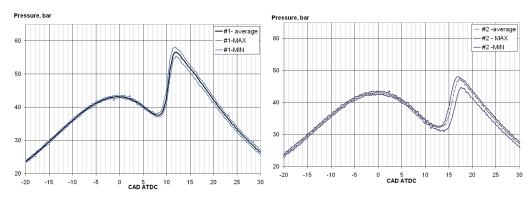
*Figure 4.13* –Cycle to cycle dispersion: average measured pressure cycle (black) and respective minimum and maximum cycle
