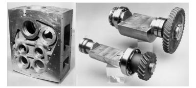
Figure 2.2 - A view of the zero vibration crankcase and balancing shafts.
