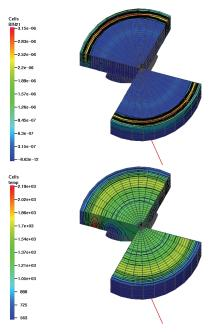
*Figure 5.17* – Upper: spatial distribution of the concentration of section BIN21- corresponding to a mean diameter of 80nm- values are displayed in ppm. Lower: spatial distribution of temperatures – expressed in K- at the same CAD value.
