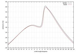
Figure 5.27 - Comparison between measured and computed pressure cycle for case in Tab 5.3.
