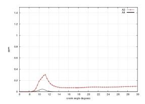
Figure 5.14 - Phenantrene (A3) and pyrene (A4) in-cylinder total concentration - ppm
