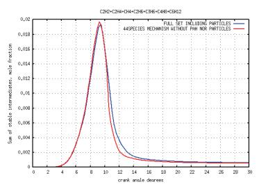
*Figure 5.3* – Sum of stable intermediates (acetylene, ethylene, methane, ethane, propilene, butane and esene) calculated with the autoignition reaction mechanism (red line) and with the full reaction set including the particle sectional model – (blue line)
