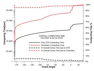
*Figure 3.2* – Fractions of computing time devoted to the CFD calculations and to the chemistry solution
