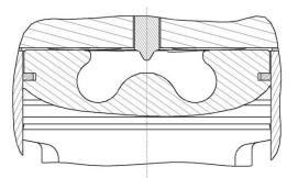
Figure 2.7 Lateral section of the piston bowl
