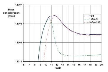
*Figure 5.18* - Predicted mass concentration due to particles with sizes in the range 1-3 nm, 3-200 nm and total mass during the main heat release phase.
