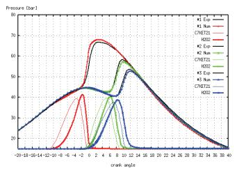
*Figure 4.11* - Experimental and numerical comparisons of pressure cycles and non-dimensional concentrations of ketohydroperoxide and hydrogen peroxide (total amount in the domain)
