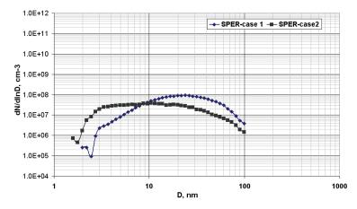
*Figure 5.30* – Number weighted particle size distribution measured by DMA in the two operative conditions
