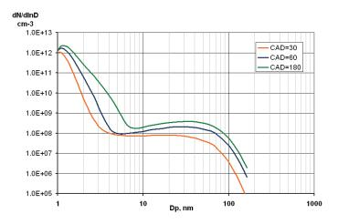
*Figure 5.23* – Size distribution function predicted at three values of the crank angle, 30, 60 and 180 degrees after the top dead centre.
