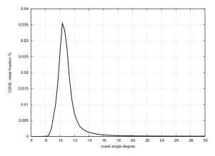
Figure 5.11 - Acetylene (C2H2) in-cylinder total concentration -mole fraction, percentage.
