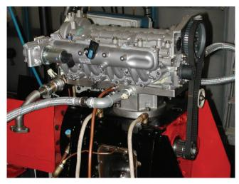
been characterised by a modular structure: the crankshaft, the cylinder and cylinder head can be changed keeping the same crankcase. Figure 2.1 shows a general view of the engine.
