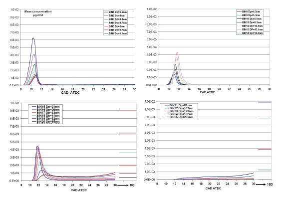
*Figure 5.15* – Mass concentration of the classes of particles against crank angle degree: the classes are grouped according to their different formation dynamics
