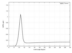
Figure 5.13 - Acenaphthylene (A2R5) in-cylinder total concentration - ppm
