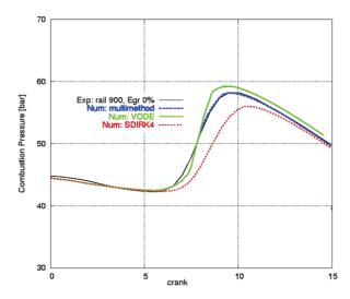
*Figure 4.5* – Pressure cycles predicted using VODE, SDIRK or the combined method, compared with the measured pressure data for case #2
