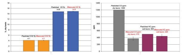
*Figure 5.10* – Comparison between concentration measured at the exhaust and in-cylinder values computed at the end of the expansion phase, for oxygen, carbon dioxide, carbon monoxide and unburned hydrocarbons.
