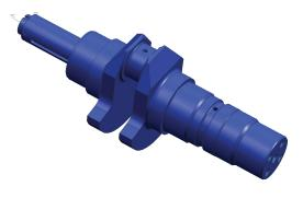
Figure 2.3 - 3D CAD view of engine crankshaft.
