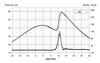
*Figure 4.17* - Comparison between measured (black lines) and calculated (coloured lines) pressure cycles varying the amount of fuel injected
