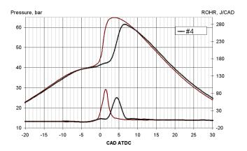
Figure 4.16- Experimental and computed pressure cycle and rate of heat release for case #4
