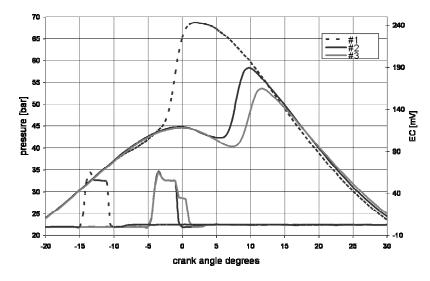
Figure 4.2 – Measured pressure and Energizing Current profiles
