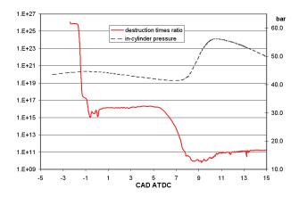
*Figure 4.3* –Ratio of maximum to minimum – among all the species- characteristic destruction time and in-cylinder pressure (on the right axis) versus crank angle, for case #2.
