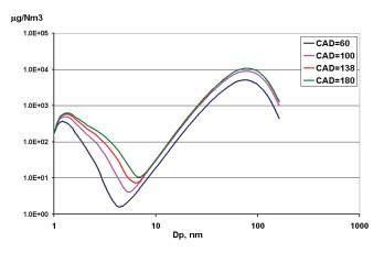
Figure 5.26 - Mass distribution function at various crank angle values
