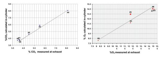
*Figure 4.19* – Comparison between calculated and measured CO<sub>2</sub> and O<sub>2</sub> concentration respectively for all the test cases
