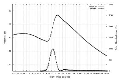
Figure 5.1 – Measured in-cylinder pressure profile and rate of heat release for case "jv15x2001"
