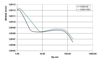
*Figure 5.28* – Size distribution function calculated at two values of the crank angle, 32 and 150 degrees after the top dead centre.
