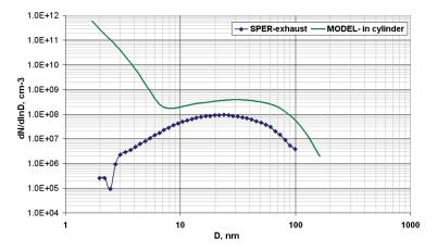
*Figure 5.31* – Number weighted particle size distribution measured by DMA compared with the simulation results at 180 CAD ATDC
