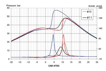
Figure 4.25 - Comparison between predicted (coloured) and measured (black) pressure cycle
