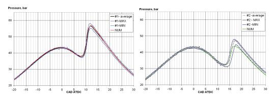
Figure 4.15 - Calculated pressure cycles and measured average, minimum and maximum cycles
