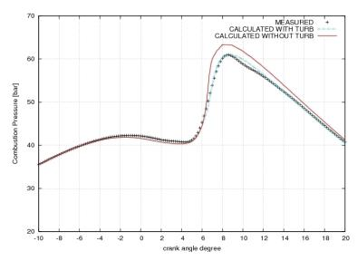
Figure 3.6 - Effect of turbulence-chemistry interaction over the predicted pressure cycle
