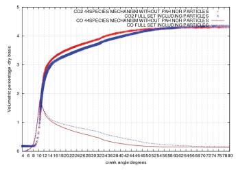
*Figure 5.4* – CO<sub>2</sub> and CO concentrations predicted by the 44 species reaction scheme (Liu, 2004) – red lines- and by the full reaction set including sectional model – blue lines.
