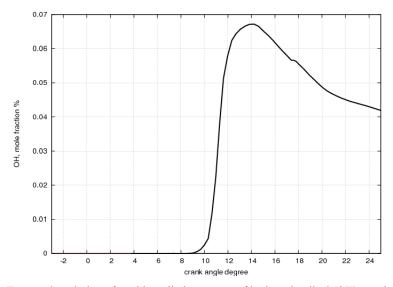
Figure 5.8 - Temporal evolution of total in-cylinder content of hydroxyl radical (OH) - mole fraction
