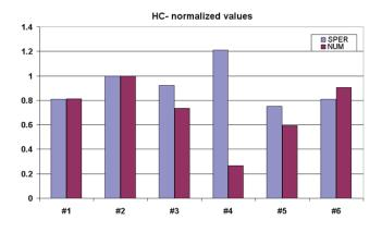
*Figure 4.21* - Comparison between normalized values of computed and measured unburned hydrocarbons for all the test cases
