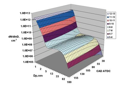
*Figure 5.24-* Predicted temporal evolution of the aggregate size distribution function between 30 and 180 CAD ATDC
