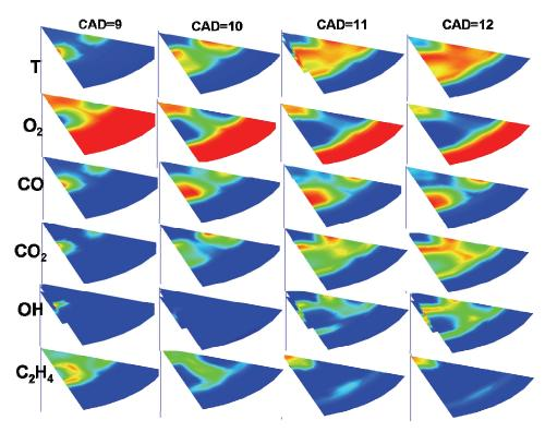
*Figure 5.9* – Comparison of the spatial variation of temperature, oxygen concentration, carbon monoxide and carbon dioxide (volumetric ppm) from 9 to 12 CAD ATDC
