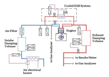
Figure 2.9 - Scheme of intake-exhaust line layout
