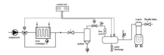
Figure 2.8 – External compressor for supercharging
