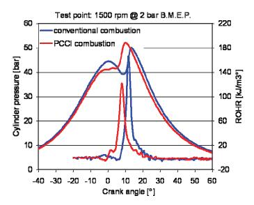
Figure 1.3 - Comparison between PCCI and conventional combustion
