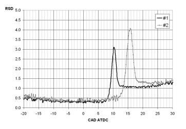
Figure 4.14 - Relative standard deviation versus crank angle for cases #1 and #2
