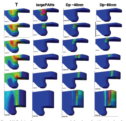
*Figure 5.16*- Evolution of temperature, soot precursors and of two classes of particles at six values of the crank angle: 10-11-13-21-30-60 CAD ATDC. Temperature- first column- varies between 800K (blue) and 2770K (red).
