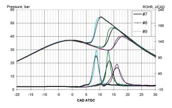
*Figure 4.24* – Predicted (coloured) and measured (black) pressure cycles for test cases with different start of injection time
