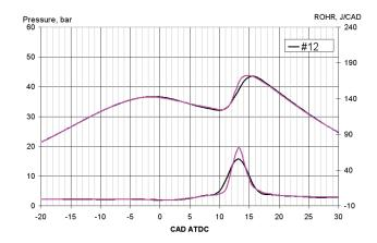
Figure 4.26 - Comparison between predicted (coloured) and measured (black) pressure cycle
