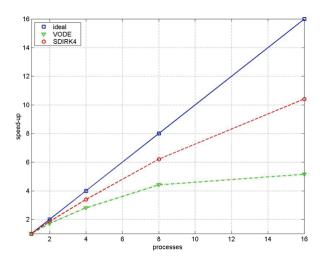
*Figure 4.8* – Speed up obtained with the two solvers using the random partitioning of the computational domain
