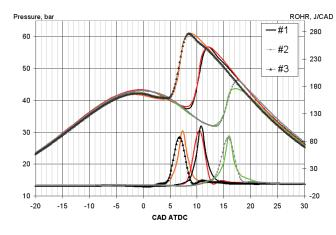
*Figure 4.12* – Comparison between measured (black lines) and calculated (coloured lines) pressure cycles and ROHR varying injection timing and EGR rate
