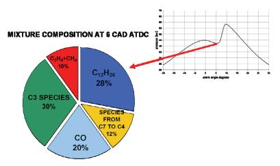
Figure 4.4 – Mixture composition calculated at 6 CAD ATDC for case #2
