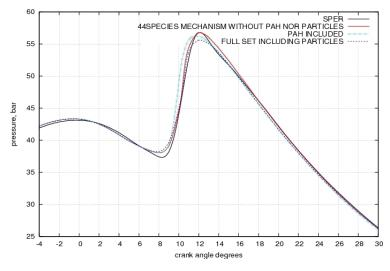
*Figure 5.2* – Effect of the reaction mechanism on the predicted pressure cycle: 44 species scheme by (Liu, 2004) – red line, addition of PAH and acetylene kinetics – green dashed line, full set including sectional model – blue dotted line. Measured values- black line.
