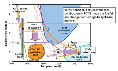
*Figure 1.2* – Equivalence ratio – temperature routes followed during conventional and PCCI combustion. (Source M. Potter, GM, DEER2006)
