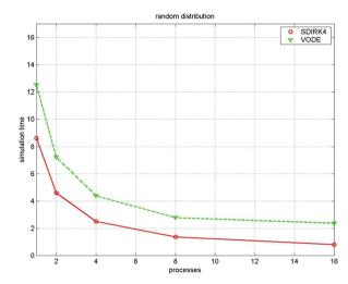
*Figure 4.6* – Hours of simulation time employed to calculate from -5 CAD to 40 CAD ATDC for the tested solvers
