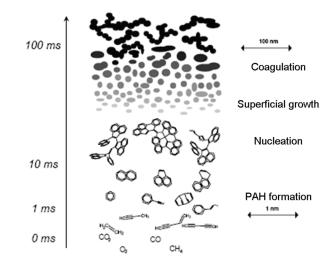
*Figure 1.6* – Particles formation mechanism adapted from (Bockhorn, 1994)
