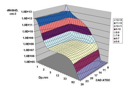
*Figure 5.21-* Predicted temporal evolution of the aggregate size distribution function between 8 and 30 CAD ATDC
