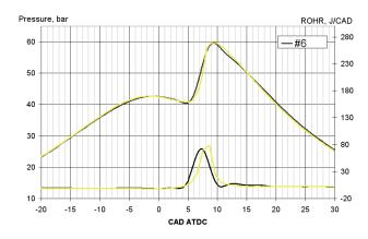
*Figure 4.18* - Comparison between measured (black lines) and calculated (coloured lines) pressure cycles varying the engine speed
