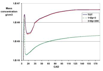
*Figure 5.19* - Predicted mass concentration due to particles with sizes in the range 1-3 nm, 3-200 nm and total mass during the expansion phase.
