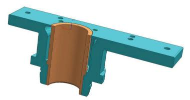
Figure 2.4 – 3D CAD view of the external block and internal cylinder.
