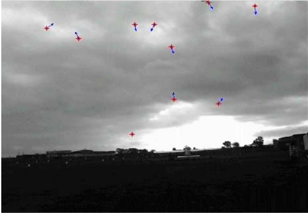
Figure 13 – Multiple false alarms in critical illumination conditions
