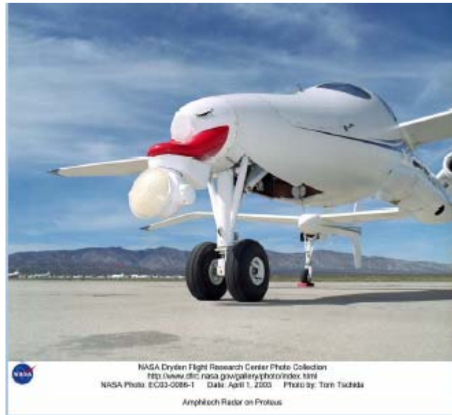
Figura 3 – Nose radar on-board Proteus
