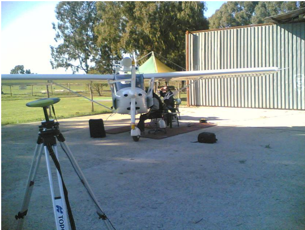
Figure 2 - Calibration procedure: acquisition of target images and position
