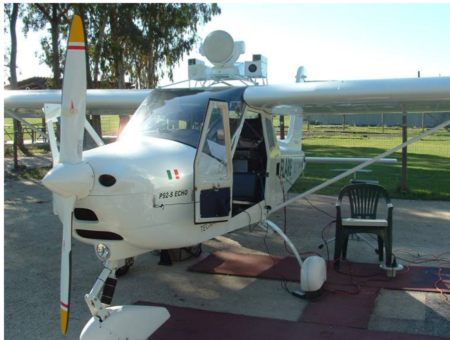
Figure 9 - Obstacle detection sensors mounted on-board FLARE
