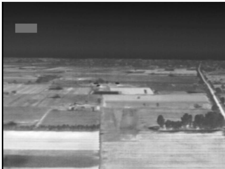
Figure 10 – Runway as seen by the infrared camera
