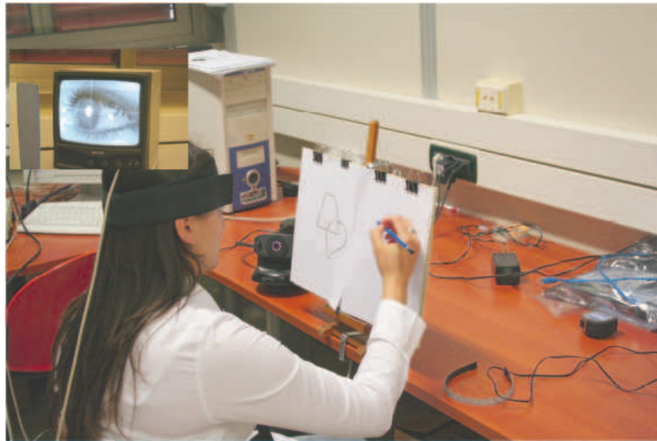
Figure 3.3: A picture of the experimental setup at the Natural Computation Lab of the University of Salerno. The inset in the upper left corner shows the control monitor for the eye camera.
