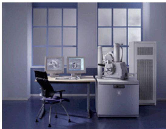
Fig. 4.2: (a) Picture of the Dual Beam Quanta 200 3D; (b) Schematic view of the relative position of columns and sample. Taken from [7].
