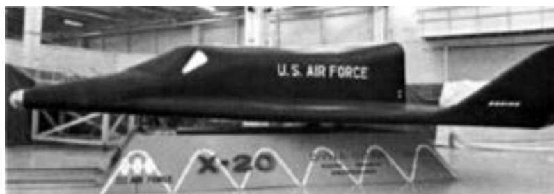
Figure 1-3. X-20 Dynasoar prototype configuration.
