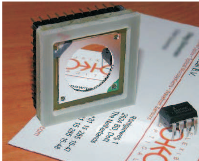
Figure 4.9: Micromachined membrane deformable mirror produced by OKOtech.
