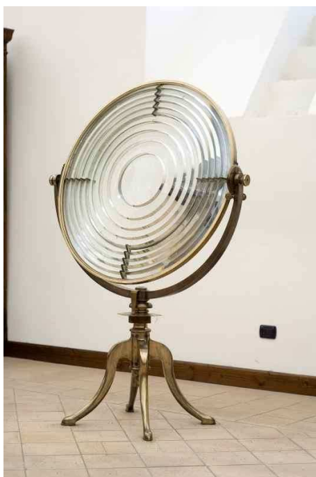
Fig. 9 Large Fresnel Lens H. Lepaute, Paris 1845
