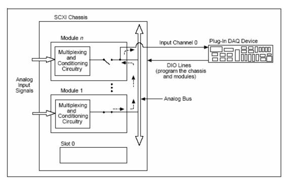
Figure B-1: SCXI signal routing.
