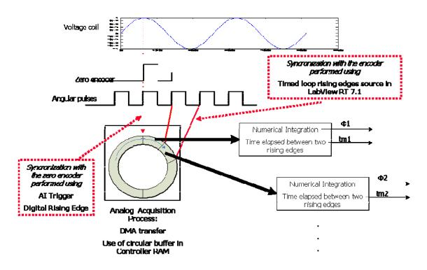
Figure III-3:Working principle of the PXI numerical integrator based on interrupt
