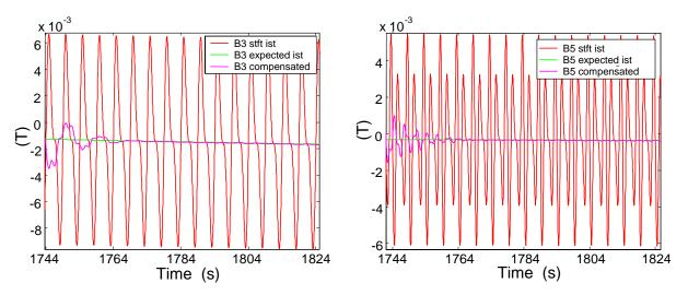
Figure IV-19: B3 and B5 compensated by demodulation and instantaneous coefficient evaluated with STFT for a coil rotating at 10s period starting from 1724 s.
