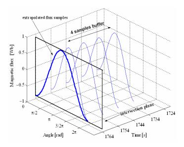
Figure IV-20: Representation of the extrapolation-based method
