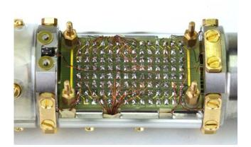
Figure II-13: The electronic connection card containing 112 points of plugs.
