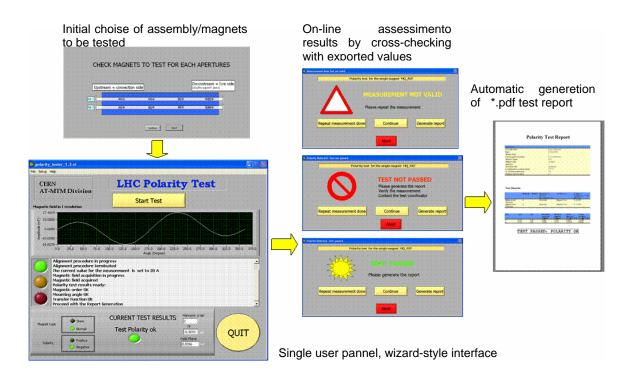
Figure VI-16: Polarity test LabView User interfaces.
