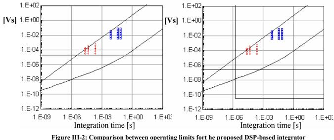
Figure III-2: Comparison between operating limits fort he proposed DSP-based integrato (on the right) and the PDI integrator (on the left), for an input gain of 1.
