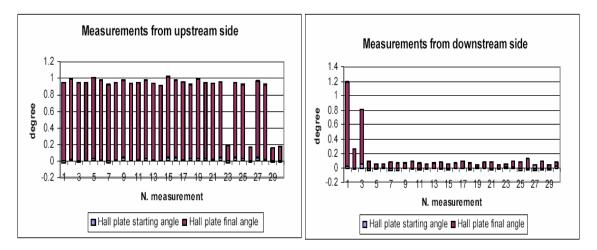
Figure VI-11: Initial and final hall plate radial position in 30 repeated measurements from upstream and downstream side in a reference quadrupole
