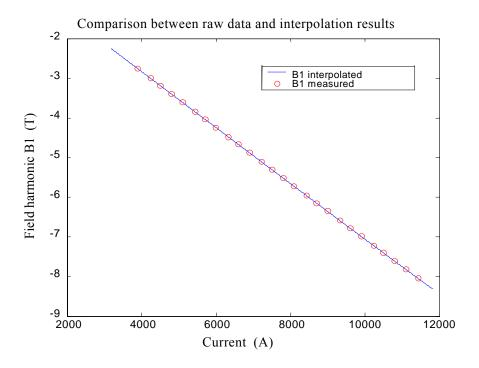
Figure IV-4: Interpolation of the harmonic coeffcient B1 on the linear current ramp at 10 A s<sup>-1</sup> of the LHC cycle.
