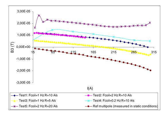
Figure IV-32: B3 measured in static conditions and in dynamic at different ramp rates and coil speeds
