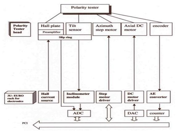
Figure VI-5: General scheme of the hardware modules used
