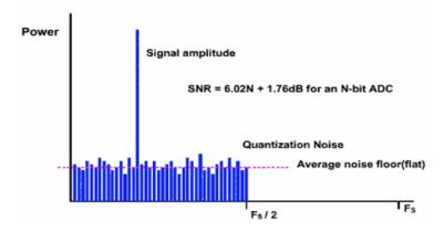
Figure V-31: Power spectrum of a pure sinusoidal tone. sampled at Fs sampling frequency
