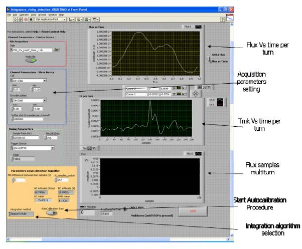
Figure III-6: PXI integrator User Interface
