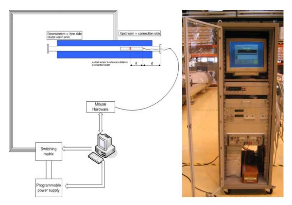
Figure VI-14: Automatic polarity test bench.
