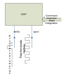
Figure III-34: The DSP interrupt system used to synchronize the integration in time domain with the trigger coming from the encoder
