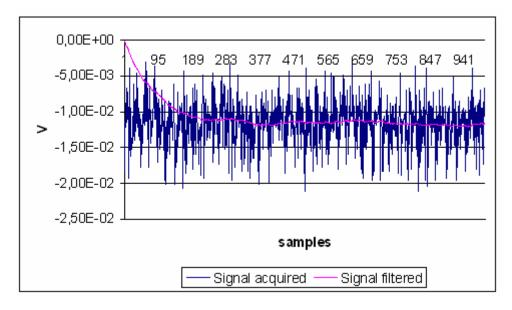
Figure VI-7: Hall plate output signal and output of the digital filter
