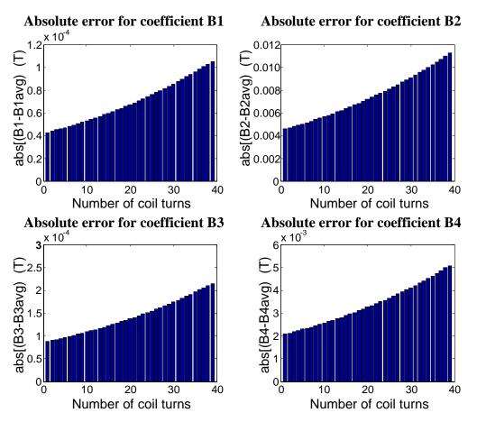
Figure IV-13: Absolute errors for field harmonics B1-B4 during an exponential current ramp. The coil rotates at 0.1 Hz frequency and the rotation starts from 1325 s.
