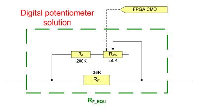
Figure III-31: Gain adjustment
