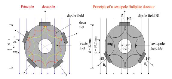
Figure II-10: Sketches of sensors used to measure the decapole (left) and the sextupole (right).
