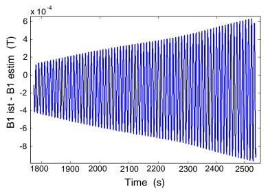
Figure IV-17: Difference between estimated and instantaneous harmonic coefficient B1.
