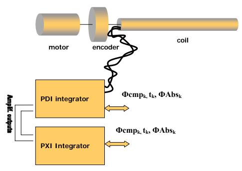
Figure III-15: Comparison between PDI integrator and PXI integrator- Experimental setup
