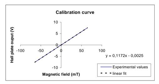
Figure VI-8: Calibration curve of the hall plate used in the instrument prototype
