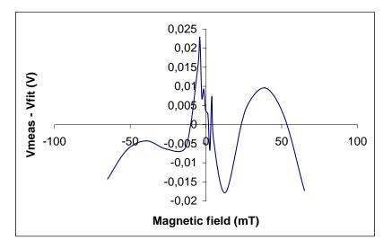
Figure VI-9: Hall plate non linearity versus the field
