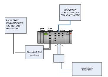
Figure V-7: Compensation cards test bench
