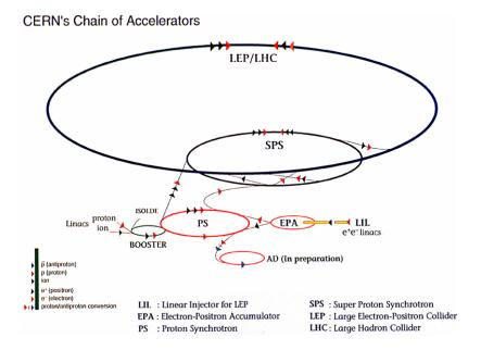
Figure I-2 The CERN accelerators structure from the beam production trough different acceleration steps up to the largest accelerator the LHC.
