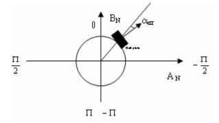
Figure VI-13: Angle error in the hall plate mounting
