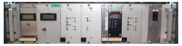
Figure VI-6: The front panel of the polarimeter electronic rack. (from left to right: the voltmeter for the tilt sensor, 50 mA hall plate supply, and, finally the power supplies for rack, DC motor, tilt sensor, stepping motor.
