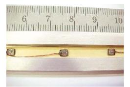
Figure II-12 Axial unpackaged Hall Plates from AREPOC, type HHP-NU used in the existing Hall detector.
