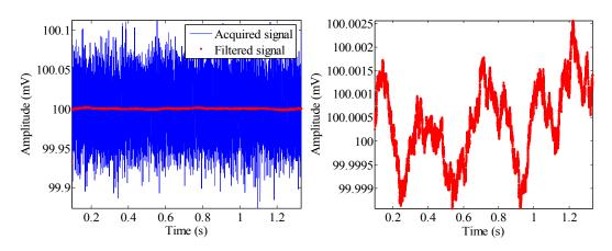
Figure V-36:Signal filtered with a 1500 samples moving average filter
