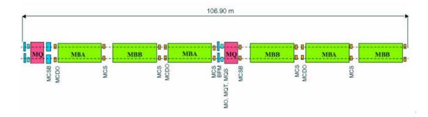
Figure I-11 Scheme of the LHC cell. Each cell includes main bending dipoles, main focusing quadrupoles, and a full correction scheme, featuring sextupoles, octupoles and decapoles.
