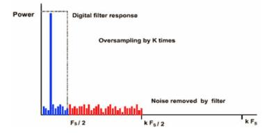
Figure V-32: Effect of the oversampling on the quantization noise
