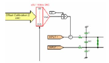
Figure III-29: The DAC based Offset calibration
