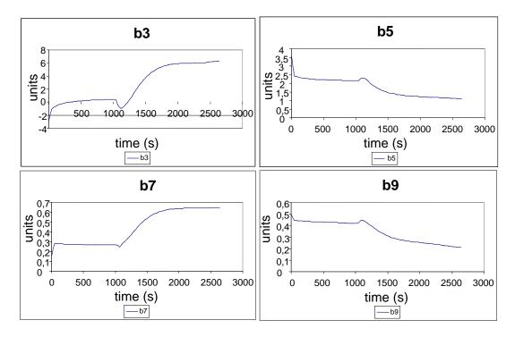
Figure IV-8: Coefficients b1,b3,b5,b7 for all the LHC cycle ramp up ( amplitude is expressed in unit in order to show the snapback phenomena at 1000 s).
