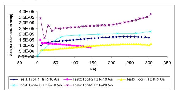
Figure IV-31:Absolute errors between B3 values measured at different current ramp rates and coil speeds and the B3 values at the same current measured in static conditions
