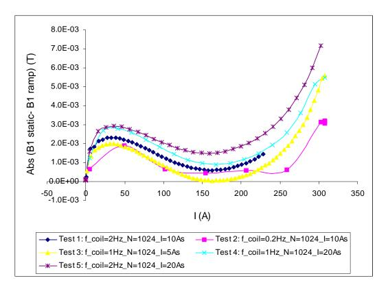
Figure IV-30: Absolute errors between B1 values measured at different current ramp rates and coil speeds and the B1 values at the same current value and measured in static conditions.
