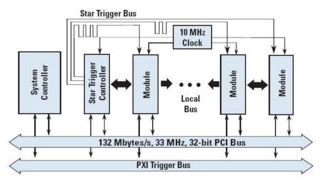
Figure A-2: PXI Timing and Triggering Buses. PXI combines industry-standard PC components, such as the PCI bus, with advanced triggering and synchronization extensions on the backplane.
