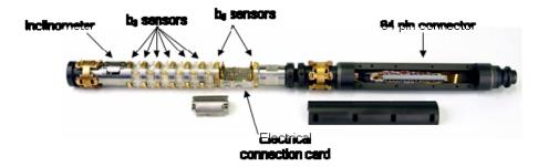
Figure V-3: CERN probe to measure b3-b5.
