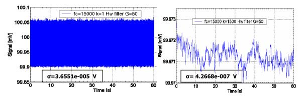
Figure V-42: The reference signal acquired without filtering (left). The same signal acquired with 1500 over-sampling factor (right).
