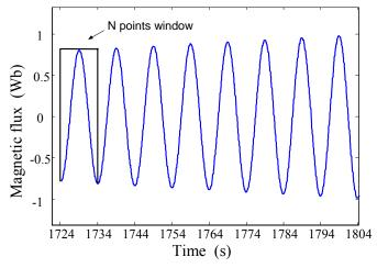
Figure IV-9: The coil rotation period is 10s during a linear ramp with 10 A  $s^{-1}$  ramp rate.
