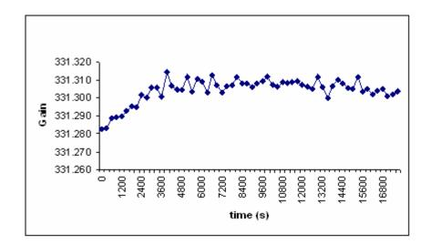
Figure V-12: Gain variation of the compensation circuit ring b3\_1.
