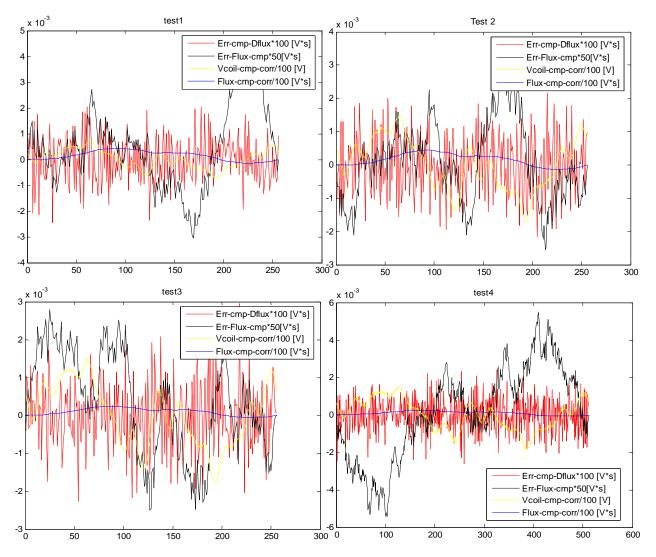
Figure III-22:Comparison between the PDI and PXI integration in all the compensated measurements performed. On the same graph the differences between the flux samples and the respective flux increments as well as the input voltage and the flux are shown.
