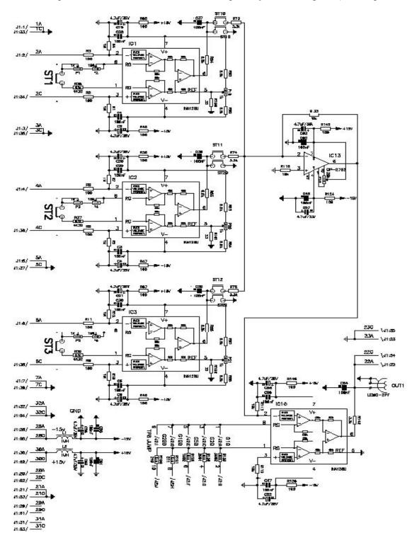
Figure V-6: A schematic draw of a sextupole compensation card.
