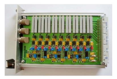
Figure V-5: Compensation card for three sextupole rings.
