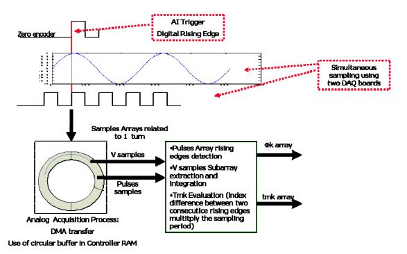
Figure III-12: Working principle of the PXI numerical integrator based on encoder signal sampling.
