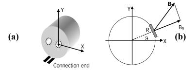
Figure VI-1: Frame of reference for the magnetic measurements: (a) sign convention and (b) radial component of the field.
