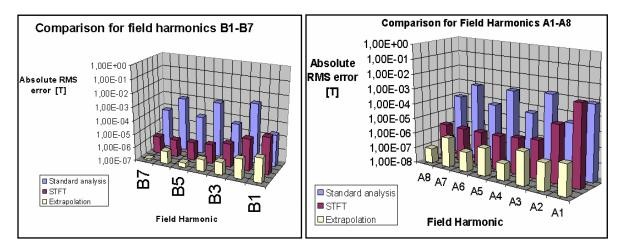
Figure IV-27: Comparison of absolute RMS errors on harmonic coefficients B1-B7 and A2-A8 for a parabolic current ramp. Coil rotation frequency is 0.1 Hz.
