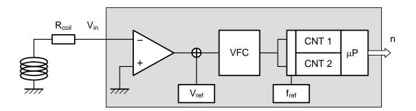
Figure II-6: Principle of the digital integrator based on voltage-to-frequency conversion
