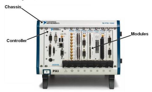
Figure A-1: A standard 8-Slot PXI chassis with an embedded system controller and seven peripheral modules
