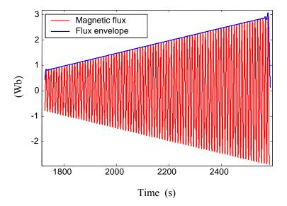
Figure IV-16: Magnetic flux and its envelope obtained by demodulation. The current is a linear ramp starting from 1724 s and the coil rotation frequency is 0.1 Hz.
