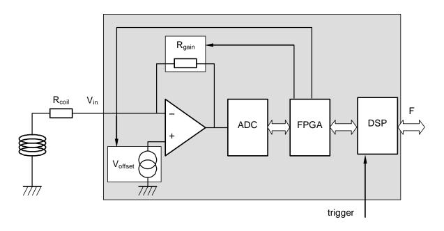
Figure III-1: Principle of the proposed digital integrator.
