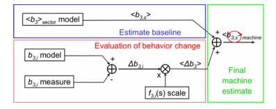
Figure I-14: Feed-forward control on the b3 harmonic
