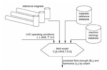
Figure I-13: Reference Magnetic System concept
