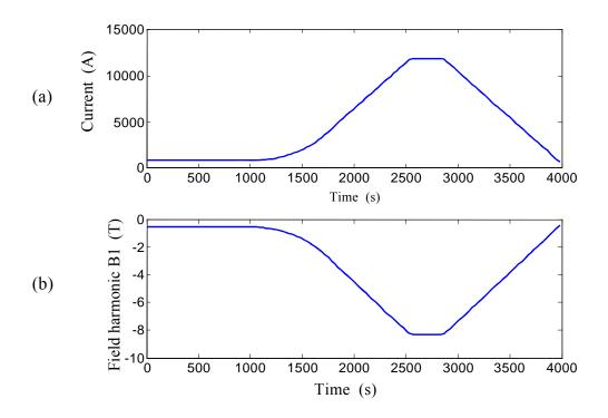
Figure IV-6: Harmonic coefficient B1 (a) and LHC current cycle (b) versus time.
