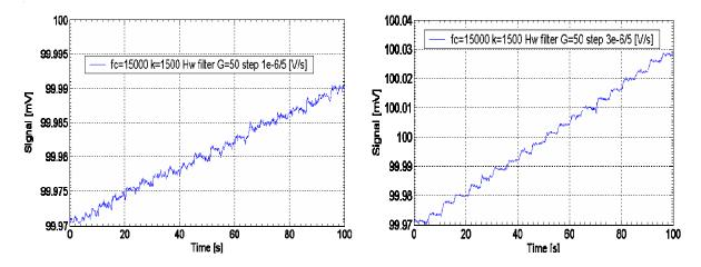
Figure V-43: On the left the reference voltage is increased of  $1\mu$ V every 5s (0.1 b3 unit) whilst on the right of  $3 \mu$ V (0.3 unit of b3).
