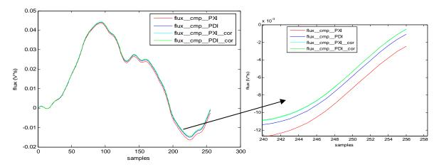
Figure III-19:Compensated flux in test 1 measured by PDI and PXI integrator with and without offset correction
