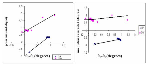
Figure VI-12: On the left relation between the phase measured on a reference normal quadrupole in repetitive measurements and the  $\theta$ F- $\theta$ I value. On the right the same main phases with the  $\theta$ F- $\theta$ I correction
