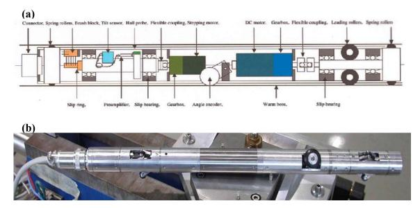
Figure VI-3: Internal layout (a) and external view (b) of the Polarity Checker probe.
