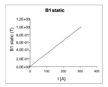
Figure IV-29: Resistive reference dipole mapping of the B1
