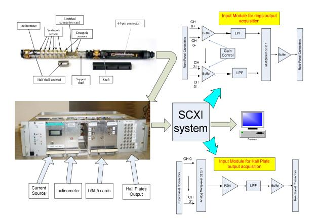
Figure V-4: b3-b5 analyzer-architecture layout.
