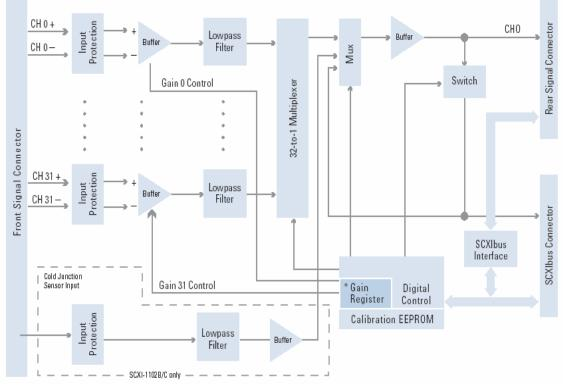
Figure B-3: Scheme of the input module for rings output acquisition
