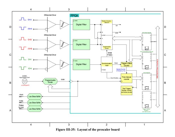
differential to single-ended mode by using standard RS-422 differential receivers. Then, two filtering stages are used to improve the noise rejection: the first, based on a Schimdt-trigger input buffer, the second, on digital filter aimed at reducing short noise spikes.
