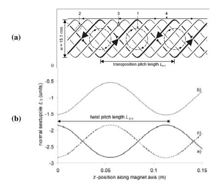
Figure I-6 (a) A schematic view of the paths followed by the strands in a Rutherford cable. (b) The longitudinal "periodic field pattern" of the b3 field component resulting from the currents loops shown in (a).
