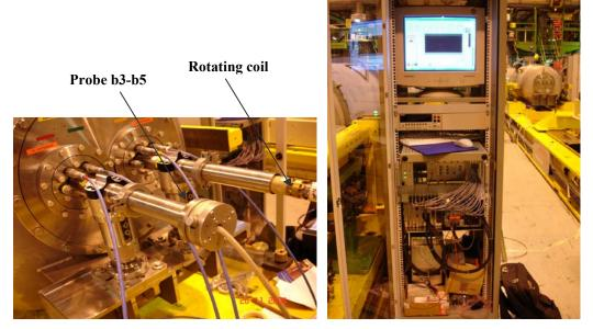
Figure V-25: Probe installation in the dipole magnet and measurement rack.
