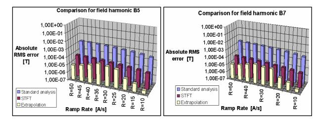
Figure IV-26: Comparison of absolute RMS error for field harmonics B5 (left) and B7 (right) using different analysis procedures. The coil rotates at 0.1 Hz frequency
