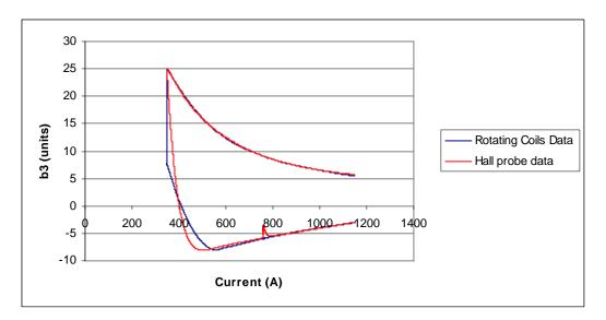
Figure V-21: Rotating coils data (blue line) and Hall probe data (red line) after the calibration
