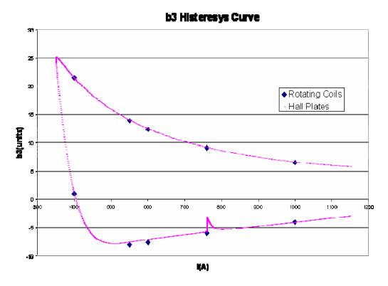
Figure V-26: comparison between rotating coils load line data (blue dots) and Hall probe data after calibration (purple line).
