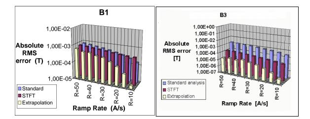
Figure IV-25: Comparison of absolute RMS error for field harmonics B1 (left) and B3 (right) using different analysis procedures. The coil rotates at 0.1 Hz frequency
