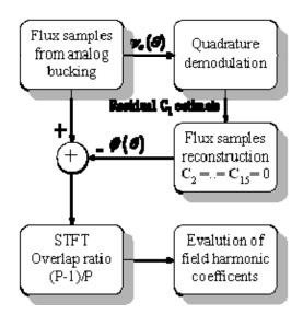
Figure IV-18: Flow diagram of the method based on quadrature demodulation and STFT.
