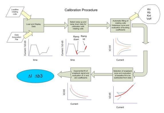
Figure V-22: Calibration and data analysis software layout
