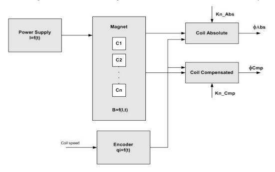
A rotating coils simulator was implemented to characterize the standard analysis, as
