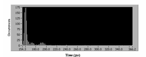
Figure III-9: Trapezoidal integration algorithm: execution time evaluation on 2500 points array- Distribution referred to 1000 executions
