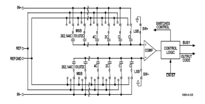
Figure III-32: Simplified schematic of the ADC 7674
