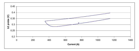
Figure V-20: b<sub>3</sub> hysteresis curve measured with the Hall probe with out calibration.
