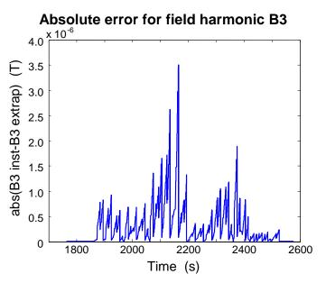
Figure IV-24: Absolute error for the harmonic B3 during the LHC linear current ramp.
