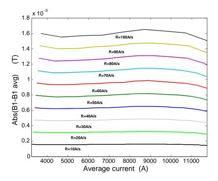
Figure IV-11: Absolute error for coefficient B1 for a coil rotating at the frequency of 0.1 Hz during a linear current ramp. The ramp rate varies from 10As<sup>-1</sup> up to 100As<sup>-1</sup>.
