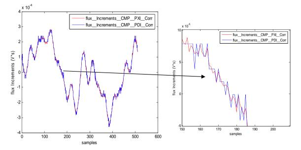
Figure III-20: Test 4 compensated flux. On the right the PDI integrator resolution limit is evident.
