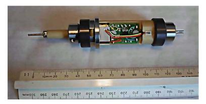
Figure VI-4: A detail of the probe assembling: the module containing the hall plate, the amplifier and the tilt sensor.
