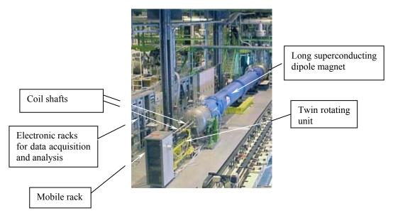
Figure II-2: Rotating coil test set-up in a long dipole magnet in the SM18 laboratory
