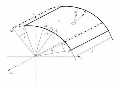
Figure II-1: Magnetic flux through a cylindrical surface.
