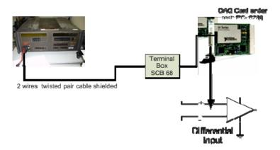
Figure V-41: Experimental setup for the testing of the 18 bit DAQ cards
