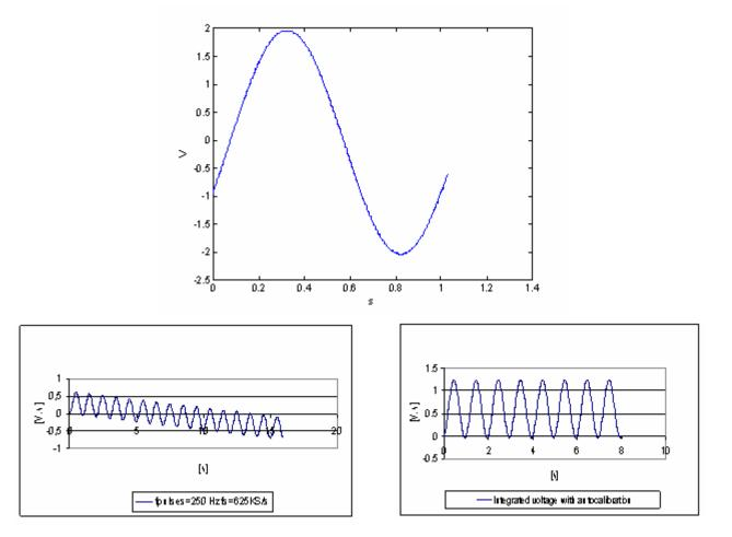
Figure III-10: Integrator autocalibration test: i)- The integrator input test signal, a sinusoidal signal A=2 Vpp, f=1 Hz (above) -The signal integrated over 8 s without offset correction (left) -The same integration performed with the autocalibration and the RT offset correction (right)
