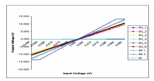
Figure V-8: Compensation circuits transfer functions.
