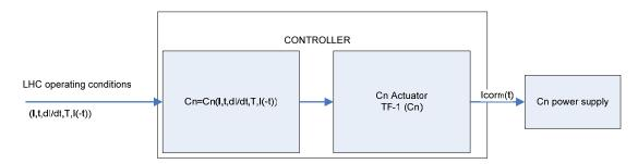
Figure I-12: Principle of the LHC multipoles errors correction without feedback
