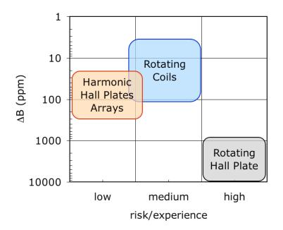
Figure 2: Scatter plot of accuracy requirements vs. the ratio of perceived risk and operator experience for the three measurements systems discussed in this thesis.
