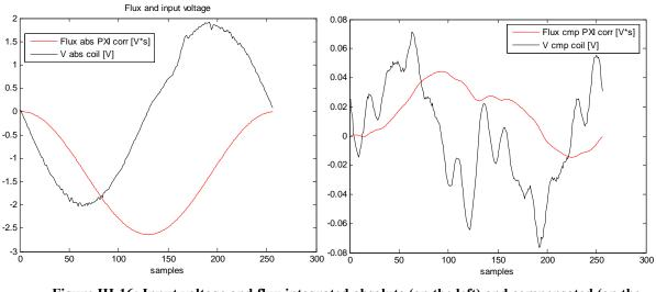
Figure III-16: Input voltage and flux integrated absolute (on the left) and compensated (on the right) for the test 1.
