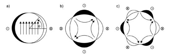
Figure I-7 Generation of pure dipole (a), quadrupole (b) and sextupole (c) fields by  $\cos(n\theta)$  current distributions with n=1,2 and 3 respectively.
