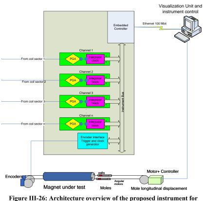
The architecture of the new rotating coils measurement system is shown in Fig. III-26.
