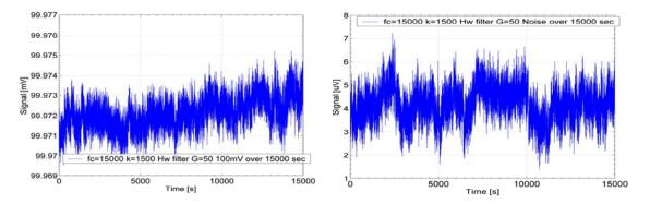
Figure V-44: Acquisitions 15000 s long with 1500 over-sampling factor of the 100 mV reference voltage on the left and with the input in short circuit on the right
