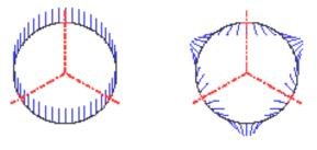
Figure II-9: Working principle of the sextupole probe. The field vectors are shown for a dipole (left) and for a sextupole (right).
