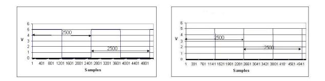
Figure III-7: The TTL signal first period measured in different acquisitions was always 2500 samples long
