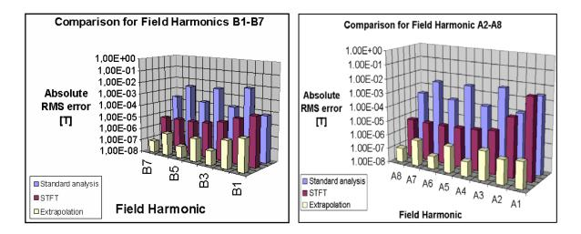
Figure IV-28: Comparison of relative RMS errors on harmonic coefficients B1-B7 and A2-A8 for a parabolic current ramp. Coil rotation frequency is 0.1 Hz.
