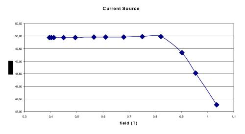
Figure V-18: current source VS field.
