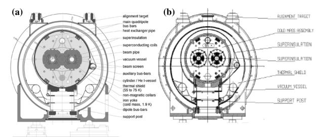
Figure I-4 (a) The cross-sections of the LHC main dipole and (b) main quadrupole, with their cryostats and overall mechanical structure.
