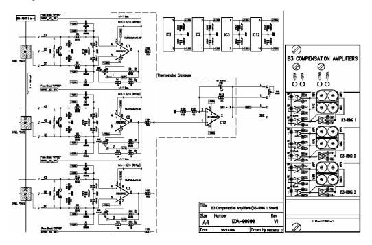
Figure V-29: Circuit layout of the new b3 compensation card and front panel.
