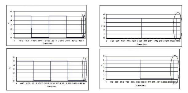
Figure III-8: The interrupt response latency time in each acquisition was almost constant and equal to 150 samples (240 us with fs=625KS/s)
