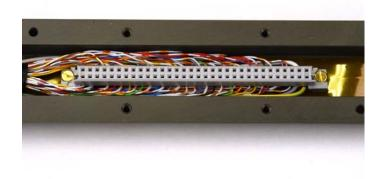
Figure II-14: The flat 64-pin connector located in the 300 mm long aluminium shaft.
