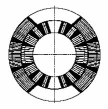
Figure I-8 Approximation of a  $\cos(\theta)$  distribution with current blocks in the LHC dipole.
