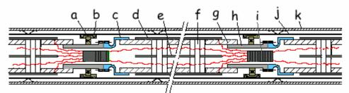
Figure II-4: Schematic assembly of a module showing the main components: (a) ball bearing, (b) brass cage with roller, (c) Ti-bellow, (d) tangential coil, (e) central coil, (f) dowel pin, (g) ceramic support, (h) SiN flange, (i) cable connector, (j) anticryostat, (k) cold bore.
