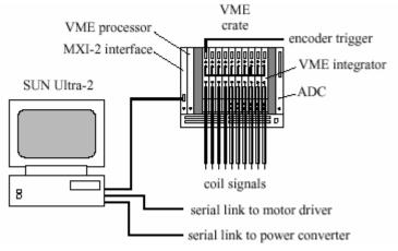
Figure II-7: Block diagram of the rotating coils DAQ system.
