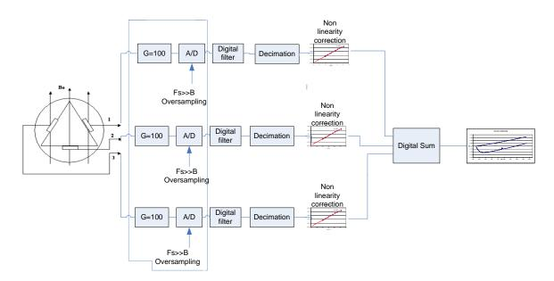
Figure V-30: digital bucking working principle.
