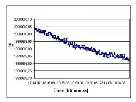
Figure III-38: Clock stability test.
