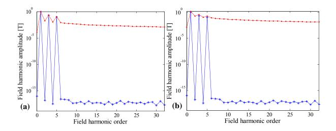
Figure IV-2: Interference on higher order harmonics due to the main field modulation with coil rotating at 0.1 Hz: imposed (blu) and estimated (red) field harmonics (a) ramp rate 10 A s<sup>-1</sup> (b) ramp rate 100 A s<sup>-1</sup>
