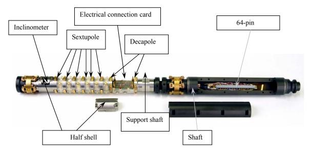
Figure II-11: The hall probe based sextupole and decapole sensor.
