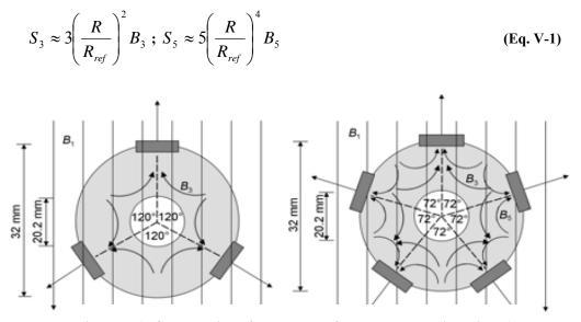
Figure V-1: Cross section of sextupole, left, and decapole ring, right (the dipole, sextupole and decapole field lines are also illustrated).
