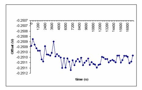
Figure V-11: Offset variation on the output of the compensation circuit ring b3\_1.
