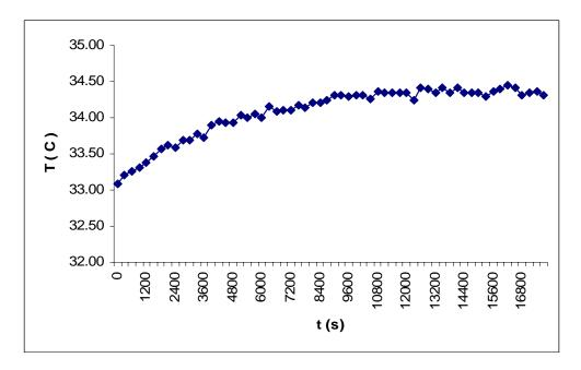
Figure V-13: Temperature chart in the electronic rack during the stability test.
