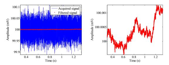
Figure V-38: Signal filtered with a 4500 samples moving average filter
