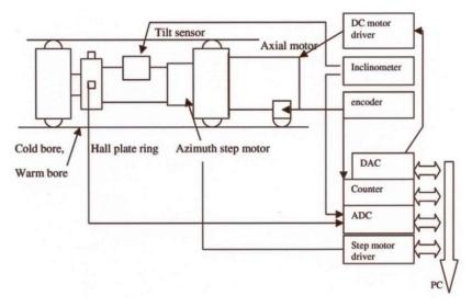
Figure VI-2: Layout of the field polarity tester.
