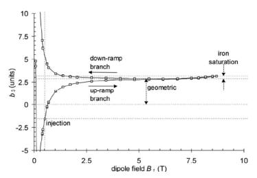
Figure I-9 Normal sextupole hysteresis cycle measured in LHC dipole model at different current levels in steady-state conditions. The currents were reached with stepwise ramp-up and ramp-down; the arrows mark the ramp directions.
