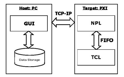
Figure III-4: Task hierarchy on the PXI target.
