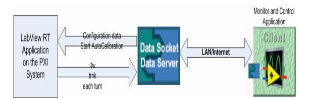
Figure III-5: Comunication layout between remote target and host computer
