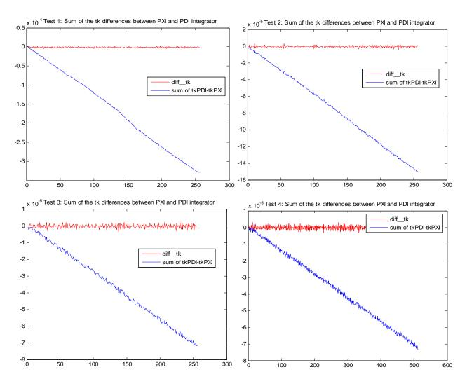
Figure III-25: Sum of the differences between the tk measured respectively with the PDI and PXI integrator in all the absolute flux measurements performed
