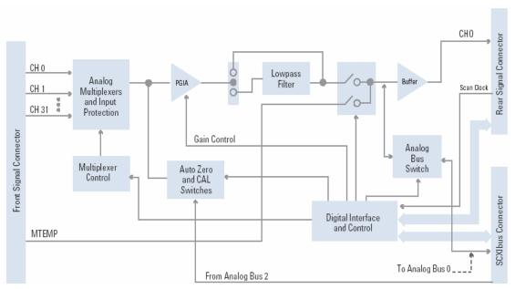
Figure B-2: Scheme for input module for Hall plates outputs acquisition.
