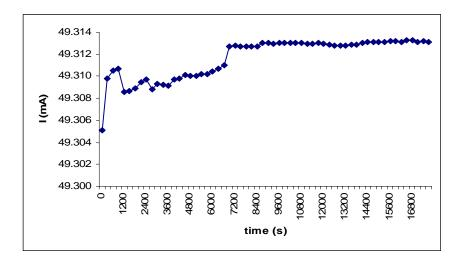
Figure V-14: Hall plate current supply the stability test in 5 h working.
