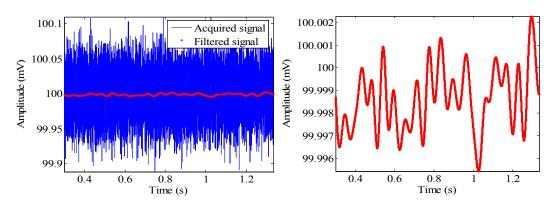
Figure V-37: Signal filtered with a 4500 samples FIR filter
