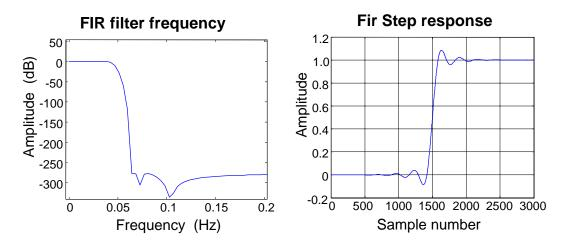
Figure IV-15: FIR filter frequency and step response.
