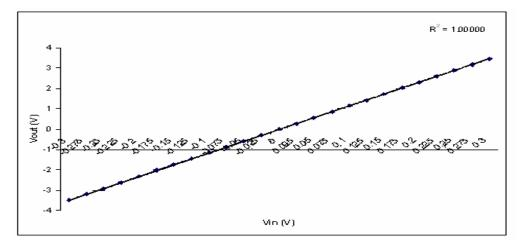
Figure V-9: Transfer function of the 1<sup>st</sup> input amplifier with a common mode input. The gain is 3.762E-4.
