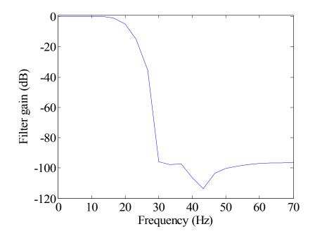
Figure V-35: Frequency response of a FIR filter at 45 coefficients designed ad hoc.
