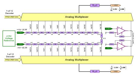
Figure III-30: Voltage reference generator.
