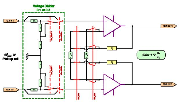
Figure III-28: Layout of the gain programmable amplifier.
