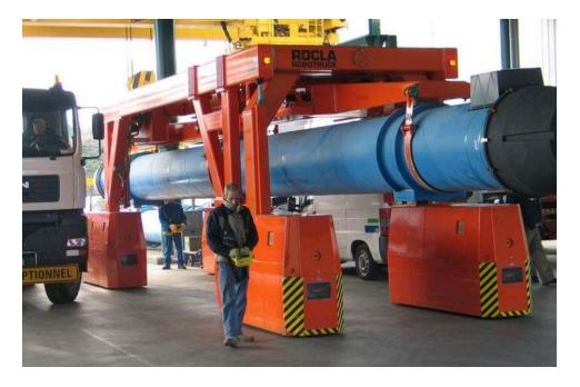
Figure I-3 A LHC dipole magnet being transported to the test benches.
