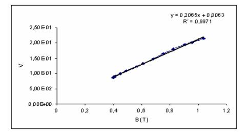
Figure V-16: First ring b3 Hall plate top transfer function
