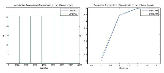
Figure III-13: Acquisition of the same TTL signal on the two input channels. On the right the perfect synchronization and the negligible interchannel delay is showed
