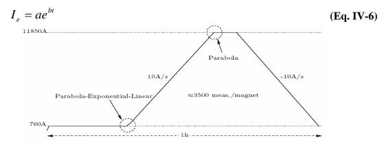
Figure IV-5: The normal LHC machine cycle (PELP).
