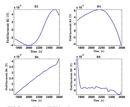
Figure IV-7: Even coefficients B2-B8 for a linear current ramp at 10A/s ramp rate starting form 1724 s.
