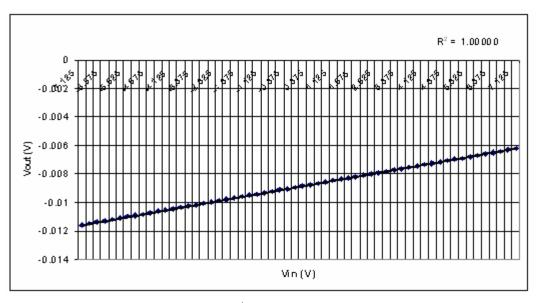
Figure V-10: Transfer function of the 1<sup>st</sup> input amplifier connected in differential mode
