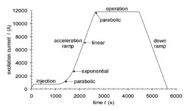
Figure I-10 The LHC current level cycle. During injection the LHC main ring will accept particles from the SPS, then a ramp-up during particle acceleration is needed to achieve the 7 TeV beam energy. At last the current is decreased back to zero.
