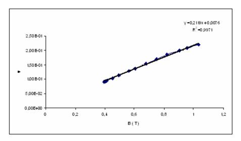
Figure V-17: Second ring b3 Hall plate top transfer function
