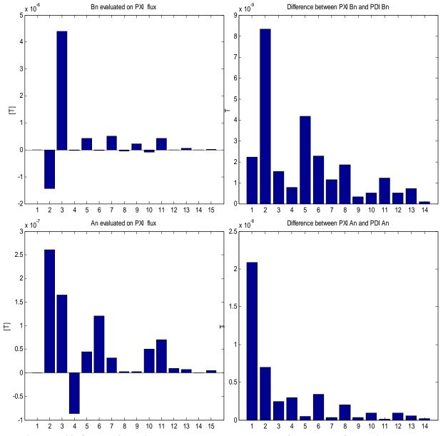
Figure III-23: On the left multipoles values measured on the PXI flux samples. On the right the differences between the same multipoles measured using the PDI flux samples and the PXI. The main field B1 is equal to 7,0822 mT with 0.1889 mT A1. The measurement is related to the test1.
