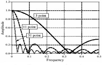
Figure V-33:Frequency response of the moving average filter
