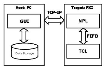
Figure V-45: Digital bucking software architecture.
