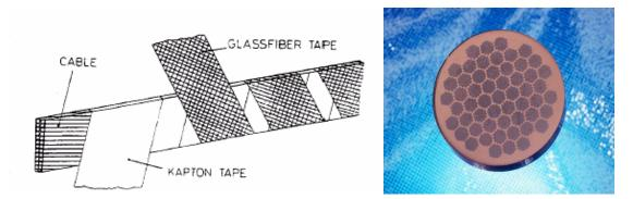
Figure I-5 On the left, Rutherford cable with Kapton and glass-fibre epoxy insulation. On the right, the cross section of an LHC dipole strand.
