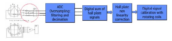
Figure V-39: Digital bucking layout implemented on the DAQ system 16 bit
