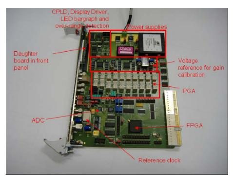
Figure III-36: Analogic front-end prototype.
