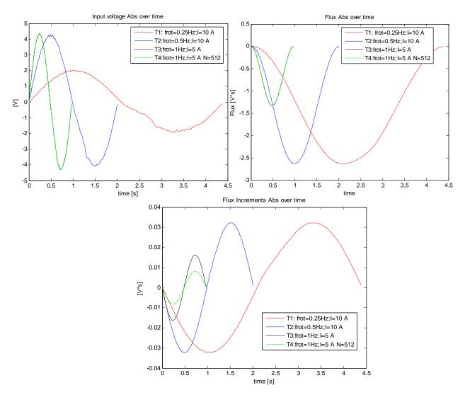
Figure III-17: Input voltage, Flux Increments and flux absolute at different coil speeds.
