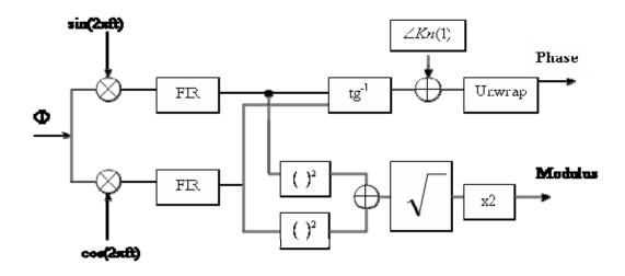
Figure IV-14: I-Q demodulation scheme.
