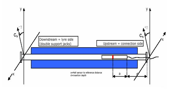
Figure VI-10: Relation between the reference systems upstream and downstream side in a main dipole
