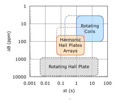
Figure 1: Comparison of the typical ranges of accuracy and time resolution for measurement systems based on rotating coils and Hall plates. In dashed lines the result of the developments described in this thesis .
