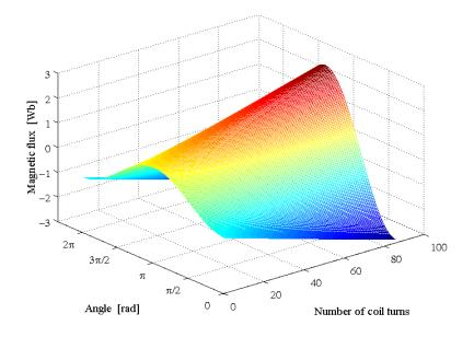
Figure IV-7: Magnetic flux evolution for different angles and several turns of the coil rotating at 0.1Hz frequency. The current ramp is linear with  $10A \text{ s}^{-1}$  ramp rate.
