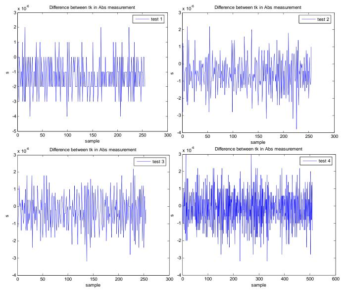
Figure III-24: Differences between the tk measured respectively with the PDI and PXI integrator in all the absolute flux measurements performed
