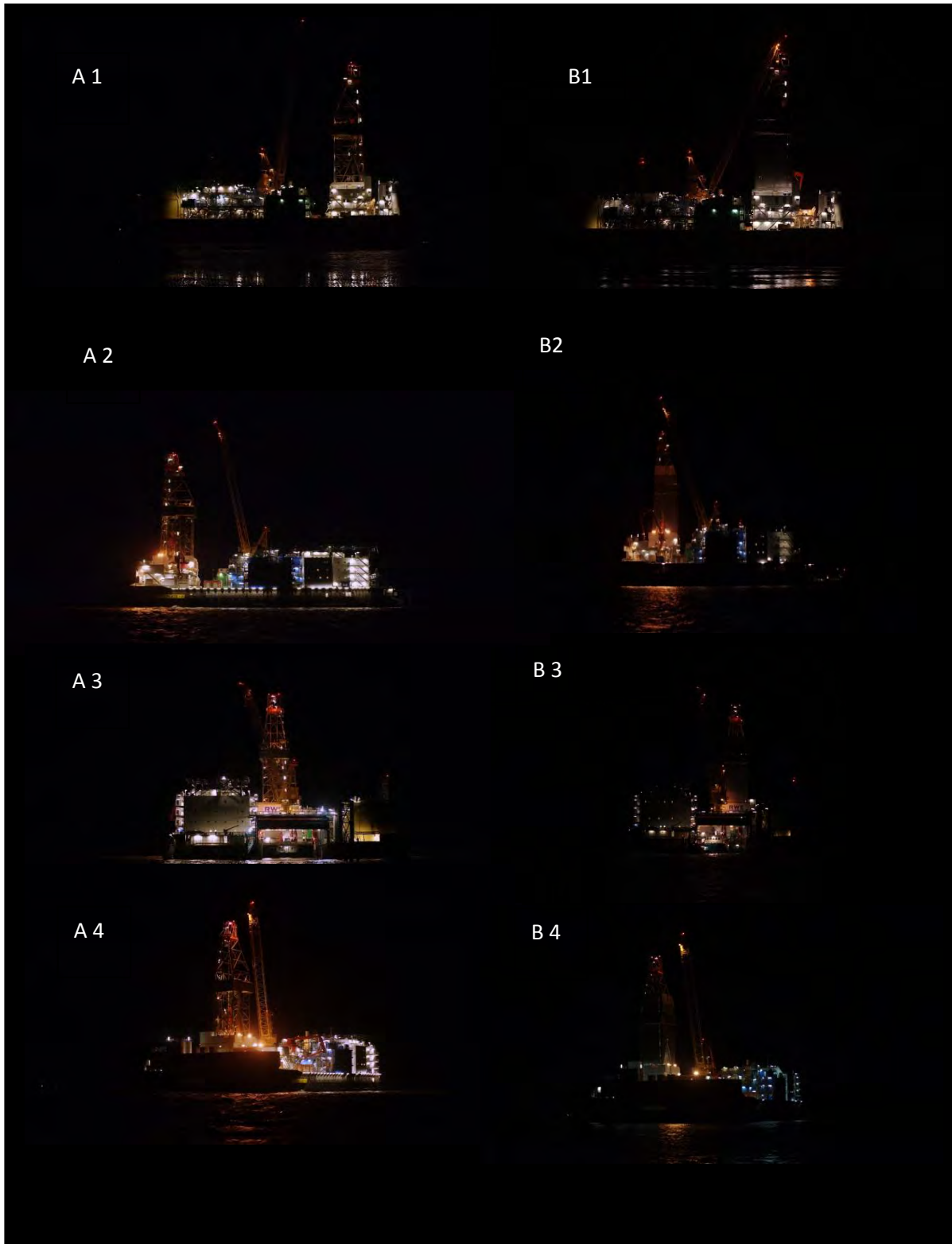
Figure 9: Comparison of lighting before (A) and after (B) from the various directions: North (1), south (2), east (3) and west (4) from a distance of 300 m (Photographs: Studio B8 on behalf of RWE Dea AG).
