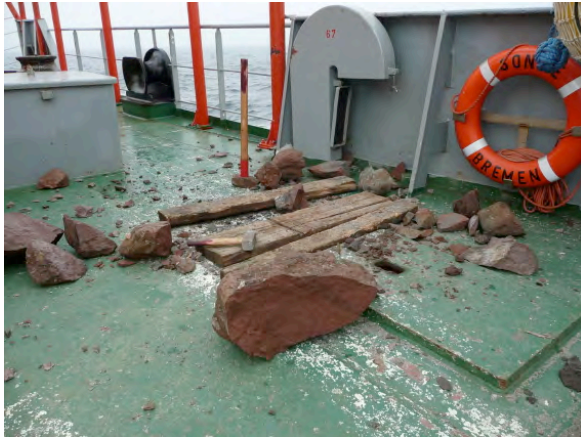
The first step of rock preparation: Crushing of large blocks on deck.
