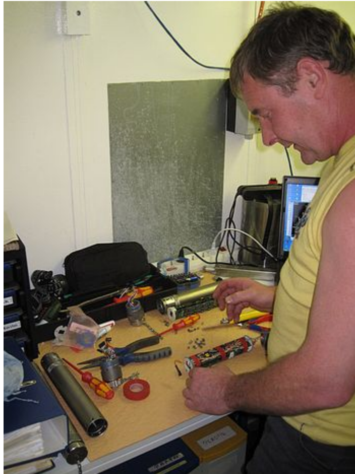
Thomas Brandt working on A/D converters for streamer segments.
