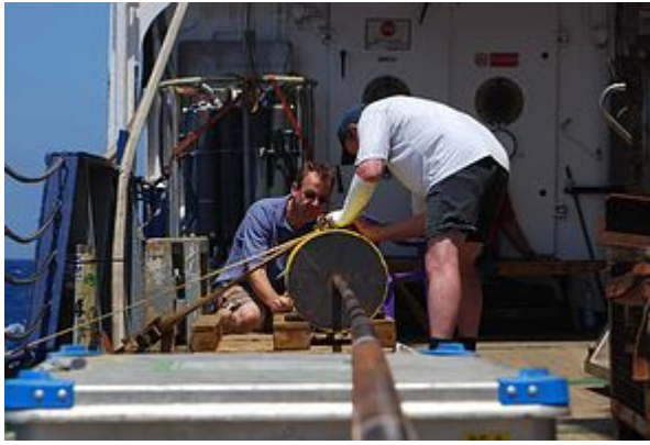
Warner Brückmann and Thomas Brandt preparing the piezometer lance
