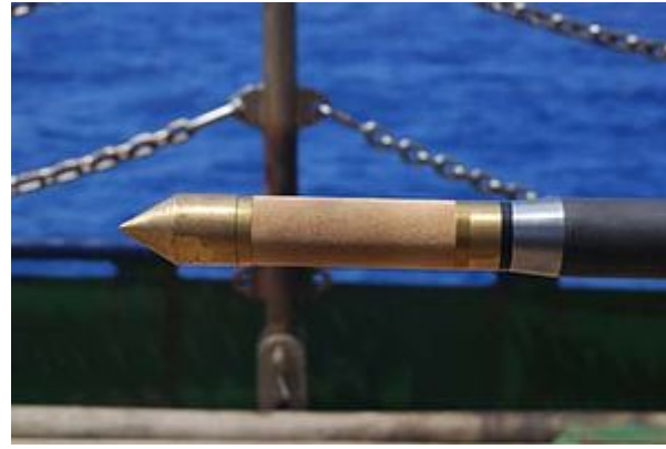
The tip of the piezometer lance is designed so that after it has entered into the sediment to depths of up to 10 m, a hydraulic connection can be made to the head of the piezometer lance, where a data logger can record changes of pore pressure for up to several years.
