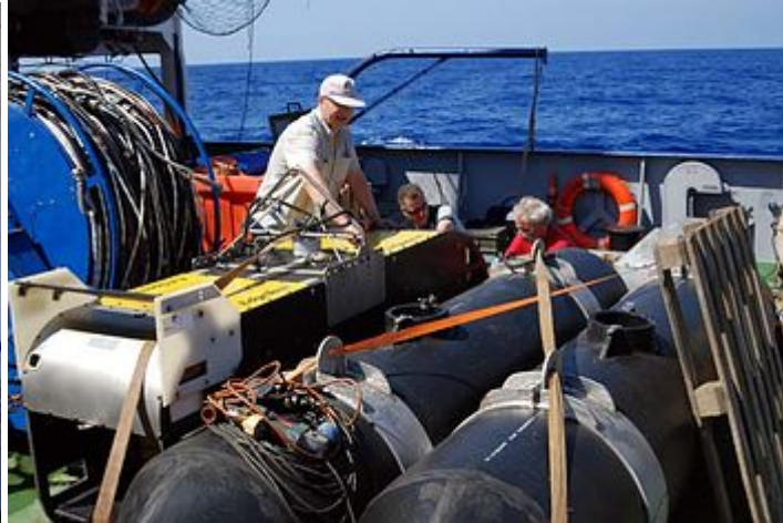
Bernd Herrmann, Ingo Klaucke and Hans-Otto Stange doing maintenance work on the side scan sonar system, which is placed on POSEIDON's afterdeck.
