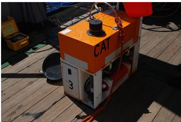
One of the autonomous CAT meters for measuring fluid and gas seeping is back on deck after having been installed at the seafloor for 8 months.
