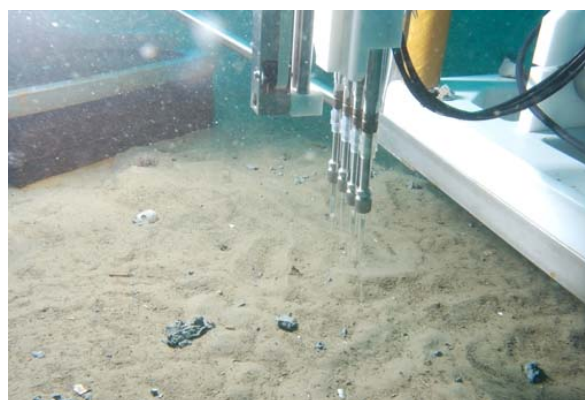
View on the microsensors deployed by the profiler in the lander. Photo: Peter Linke, IFM-GEOMAR.
