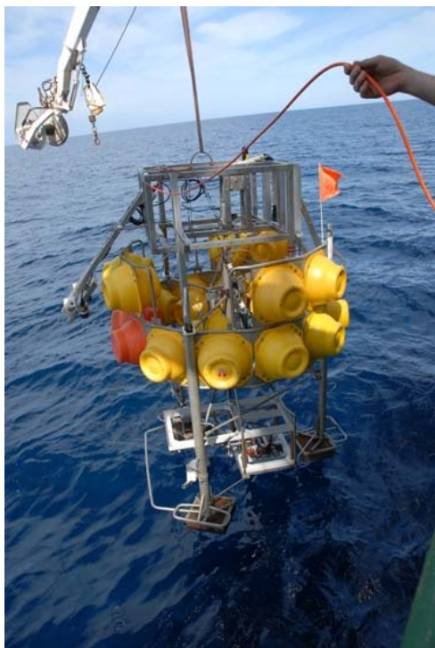
Deployment of the Profiler Lander. Photo: Peter Linke, IFM-GEOMAR.
