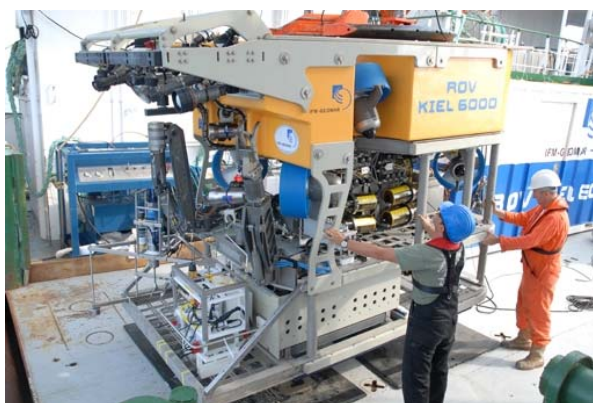
Deployment of the ROV loaded with a benthic chamber and the new Eddy Correlation System. Photo: Peter Linke, IFM-GEOMAR.
