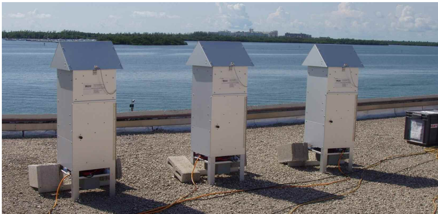
Fig. 1. Three Tisch VFC samplers, as deployed on the rooftop of the Rosenstiel School of Marine and Atmospheric Science building at the University of Miami.
