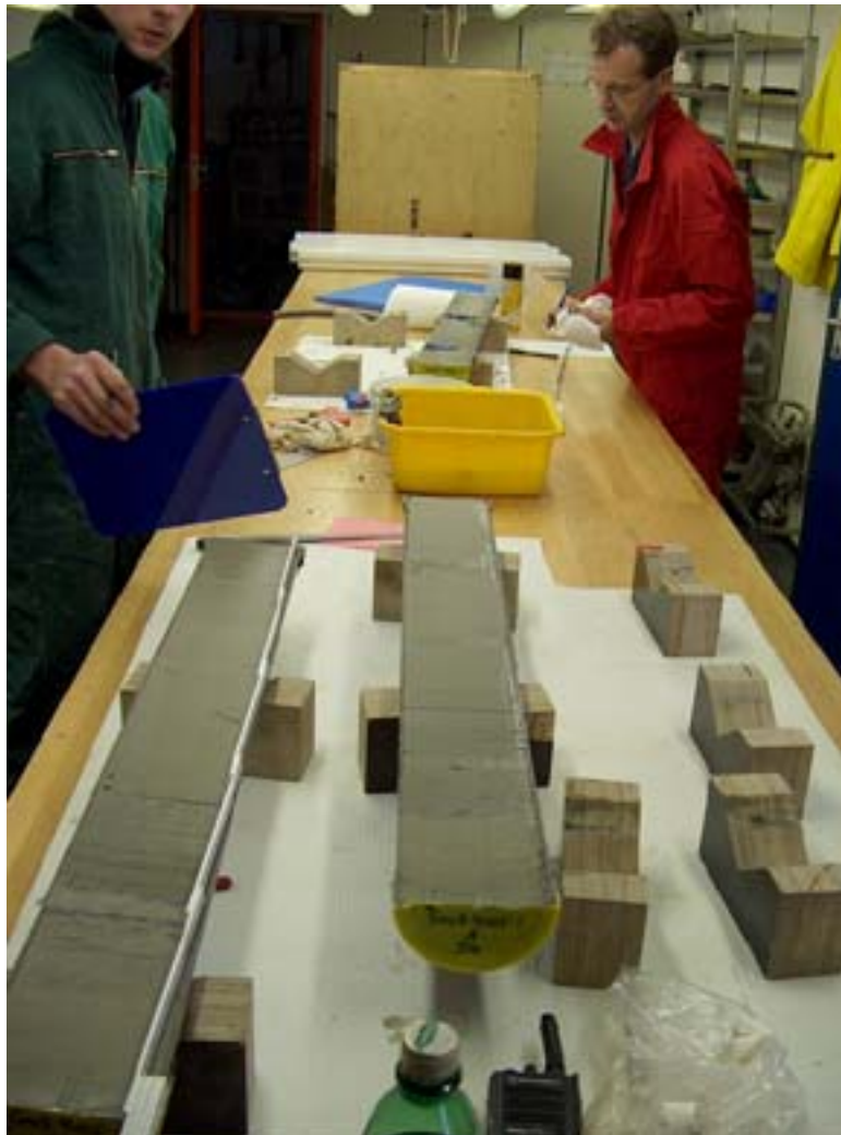
Figure 6.5. Gravity core Geob9006-1 with turbidite layers.
