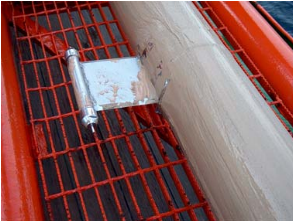
Figure 5.6 Photograph of mini-temperature logger installed on gravity core.
