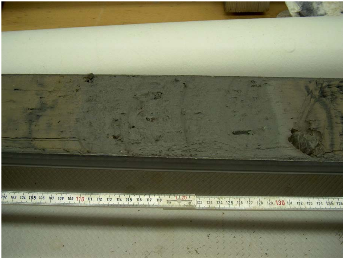
Figure 6.22. Interlayering of hemipelagic sediment (left and right portion of core) and gray mud breccia with mm-sized clasts from station GeoB 9037-1.
