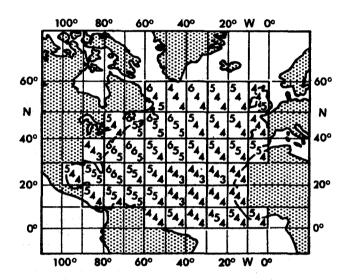
Fig. 1: The approximate base 10 log of the total number of MBT (upper left), XBT (center), and hydrocast observations (lower right) in each 10-degree square.
