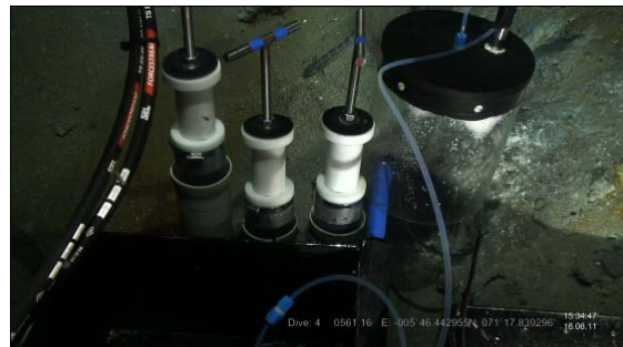
Figure 15: Collecting CO 2 bubbles from one of the Jan Mayen vent fields (© University of Bergen)
