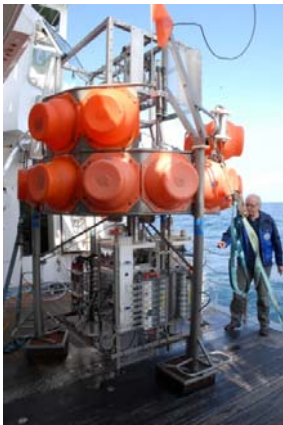
Figure 4: Video-guided deployment of a benthic chamber lander. The pCO 2 increase inside the two benthic chambers in comparison to bottom water pCO 2 reflects the background CO 2 production due to benthic respiration (© photo and image: GEOMAR)
