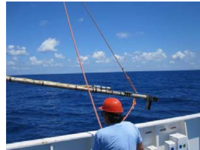
Figure 4.1.4-1: Pole-mounting of the R2Sonic multibeam transducer and external seawater pump along R/V Urania's starboard side.
