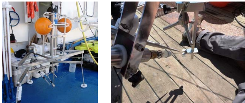
Figure 4.8.1-1. Eddy correlation instrument. Right, fast temperature and O 2 Clark electrode.
