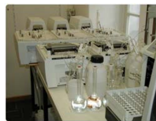
Figure 4.2-3. Segmented Flow Analyzer (Bran + Luebbe Autoanalyzer III) for nutrient analysis.
