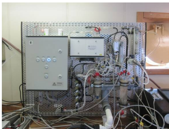
Figure 4.5.1-1: IOW Equilibrator setup installed in the wet lab of R/V Urania.
