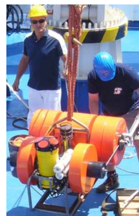
Figure 4.7.1-1. POZ-Lander with ADCP, CO 2 sensor and CTD.
