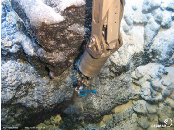
Rock sampling in 3,500 m water depth using ROV Kiel 6000. A conventional chisel held by the manipulator of the ROV turned out to be the optimal tool for rock sampling.
