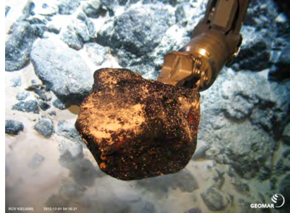
The manipulator of the ROV recovers a rock sample from the eastern flank of the Danger Island Troughs.
