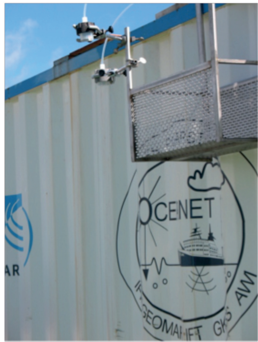
Fig. 8.1: Sampling inlets for the nitrite-coated filter sampler and continuous ozone monitor installed outside of the OCEANET container
