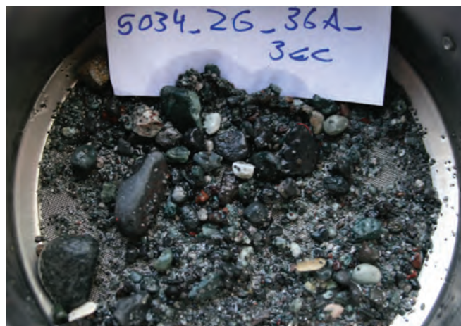
Figure 14. Washed samples of a core catcher of the basal gravel layers. The rounded nature of the gravel indicates coastal or fluvial reworking related to initial lake transgression.
