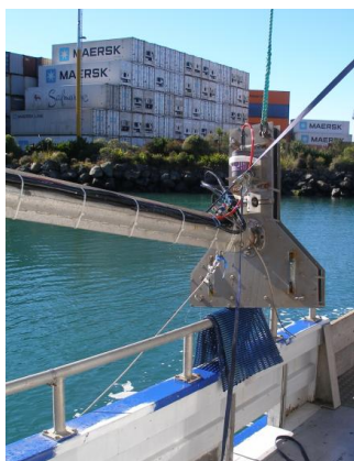
Fig. MOUNTING: Picture of the SB3050 mounted via the over-the-side-pole of Polaris II.
