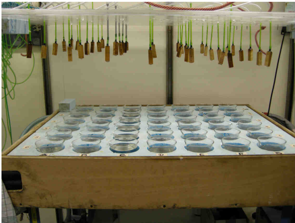
Figure 5. Temperature gradient table (Tempo) with the aeration tubes fixed in the cover plate shown. The aeration tubes were connected to the different \text{CO}_2 air mixture lines provided by the automated system.
