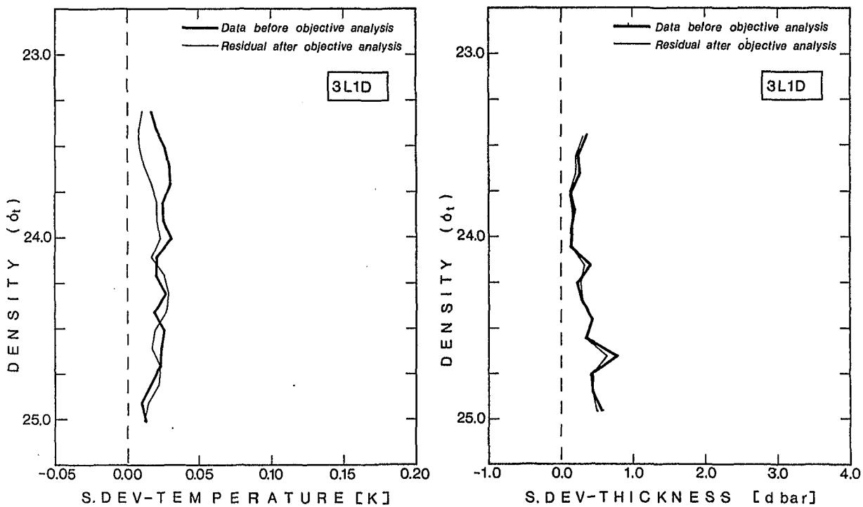
Profiles of the residual (rms error) after objective analysis onto regular grids and the standard deviation before objective analysis of potential temperature and thickness on constant  $\sigma_t = 23.30 - 25.00$  for potential temperature and  $\sigma_t = 23.45 - 24.95$  for thickness.
