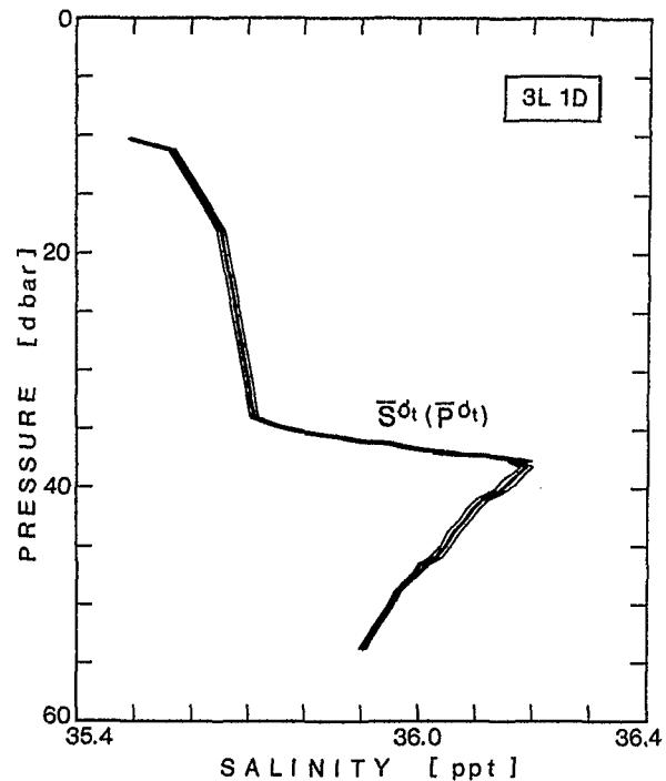
Profiles of the mean and standard deviation of potential temperature and salinity on surfaces of constant  $\sigma_t$  redrawn as functions of pressure using the mean relationship of  $\sigma_t$  to pressure.
