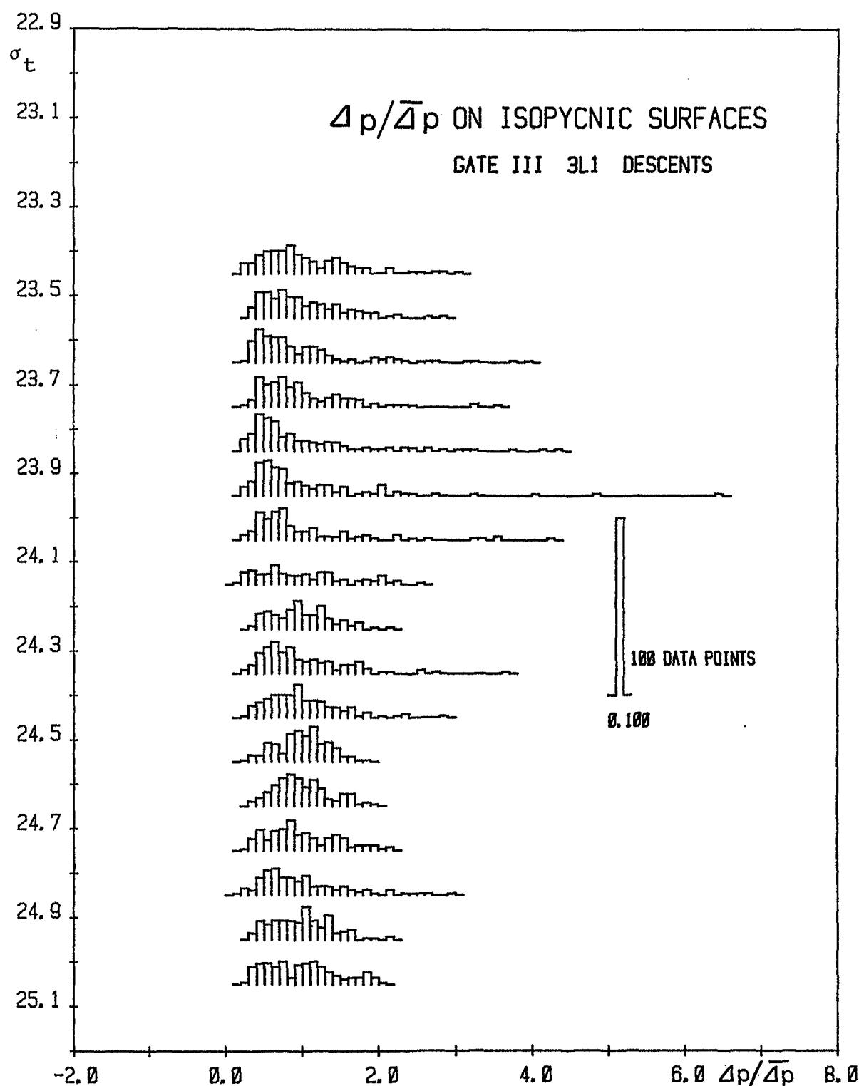
Histograms of normalized thickness on surfaces of constant  $\sigma_t$ . The thicknesses are normalized by the mean thickness on their surface to remove the effect of changes in the mean density gradient. The mean, standard deviation, skewness and kurtosis of the thickness on each surface is shown in the accompanying table.
