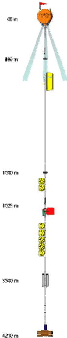
Fig. 2.7: Mooring AO_05 with full instrumentation, MMP, LongRanger ADCP, Aanderaa Rotor Current Meter, and two Seabird Microcats.
