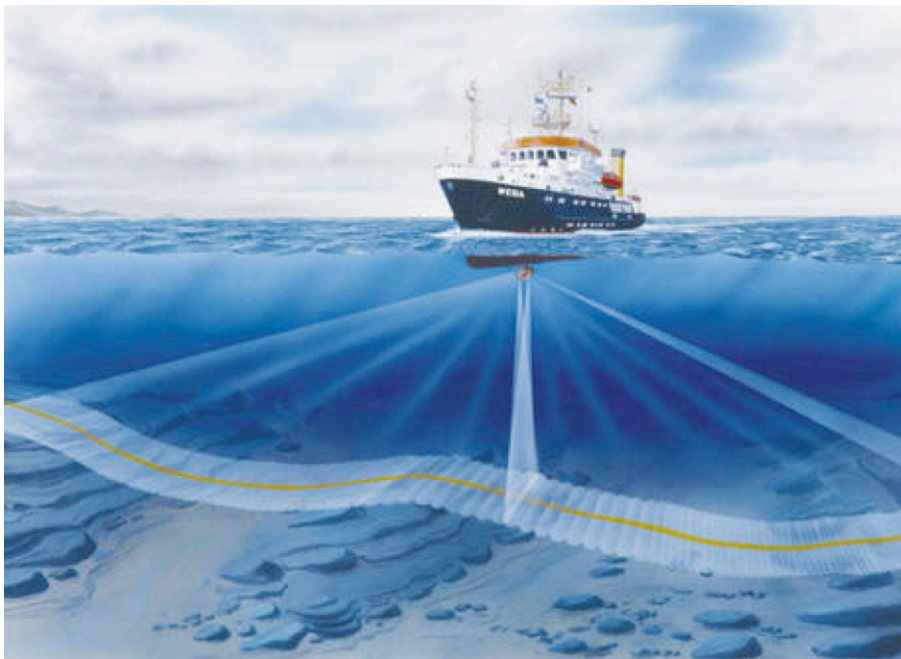
Figure 2.1: The swath of the Hydrosweep DS system from Atlas. Foto taken from: http://www.atlashydro.atlas-elektronik.com/typo3/index.php?id=2072
