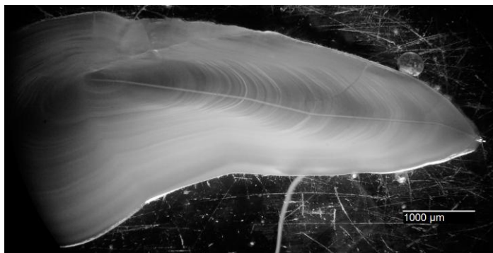
Figure IV-2: Ablation line after LA-ICPMS measurements along the growth axis of an adult cod otolith
