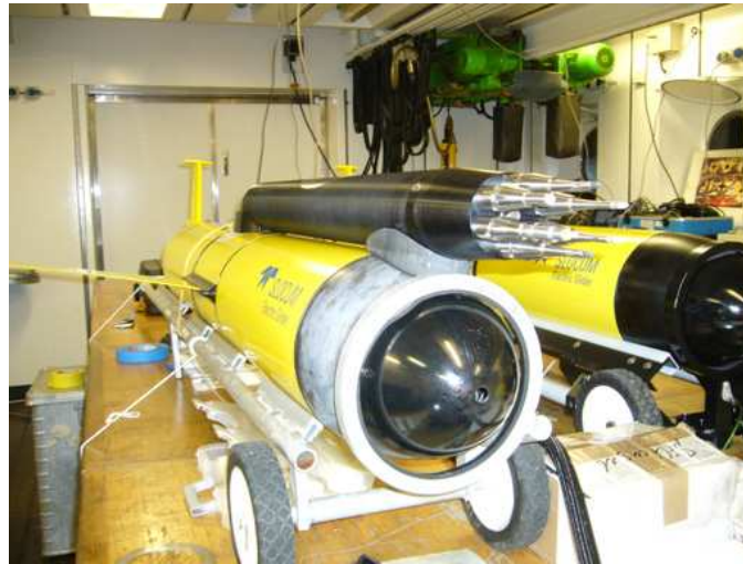
Fig. 5.6.1: Microstructure instrument package MicroRider mounted on top of a Slocum Glider
