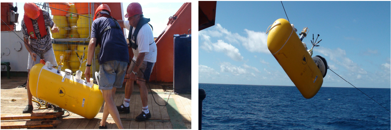
Fig. 5.4.1: Left: One of the WHOI MMPs mounted on the mooring wire – ready to be deployed. The upper stopper prevents slippage of the profiler - there exists a movie documenting the whole procedure; Right: The profiler on its way to the water. (Photos H. v. Neuhoff)
