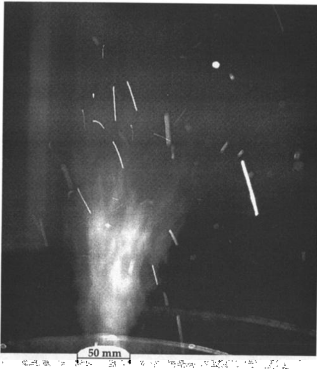
Figure 14. Photograph of a narrow fountain of strongly fragmented liquid erupted from the conduit during slug-annular flow. Liquid viscosity is \mu = 125 mPas and gas flux is M_g = 0.8 g/s.
