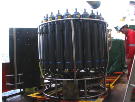
Figure 4.1 The stainless steel CTD frame with its rosette of 24 20 litre Niskin bottles.
